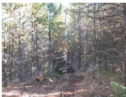
Figure 8. All-surface vehicle (ASV) with Slashbuster head, thinning young western larch stand.
