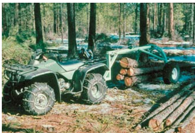
Figure 7. This ATV with a “log arch” is an example of light-duty harvesting equipment for small-diameter logs.
