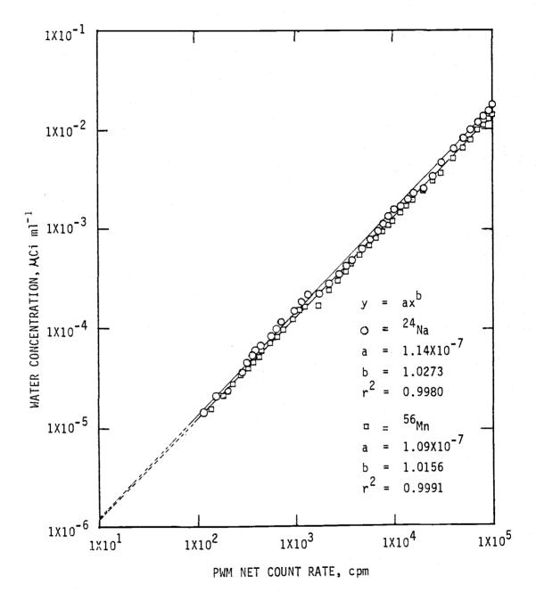
Fig. 4. Primary water monitor net counting rate in response to various water concentrations of  $^{56}$ Mn and  $^{24}$ Na under static flow conditions.
