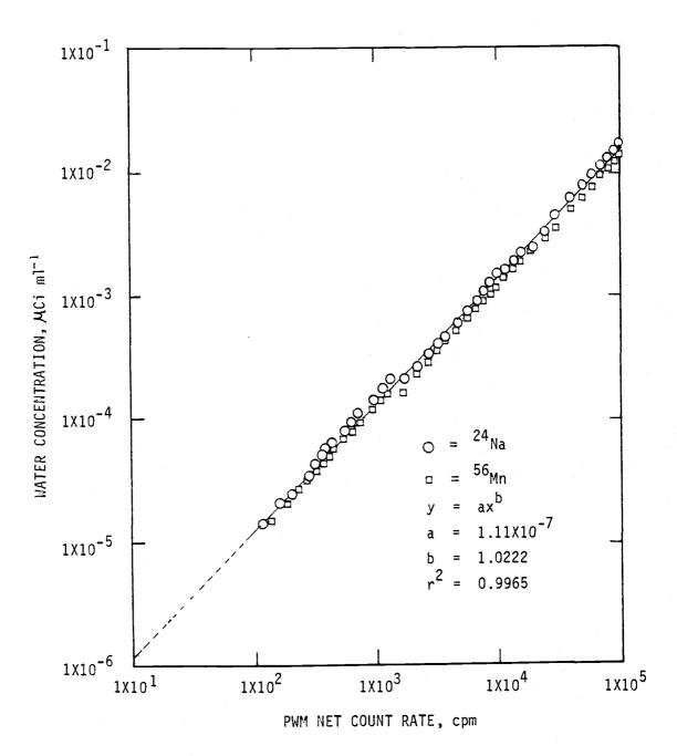
Fig. 5. PWM calibration curve based on predomonant radionuclides in the OSTR primary water (excluding <sup>3</sup>H): static flow conditions.
