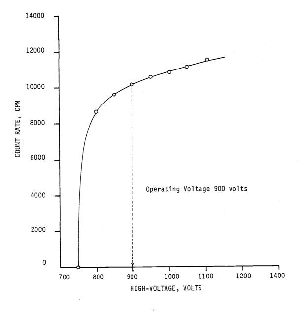
Fig. 2. Determination of Geiger tube operating voltage for the primary water monitor.
