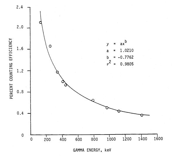
Fig. 3. Ge(Li) detector counting efficiency as a function of gamma energy.
