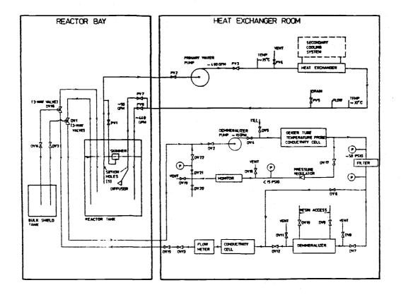
Fig. 1. General schematic of OSTR water cooling and purification system.
