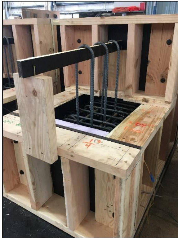
Figure 3.19: The L-shape half of a specimen containing #4 (#13M) U-bars at the correct location.
