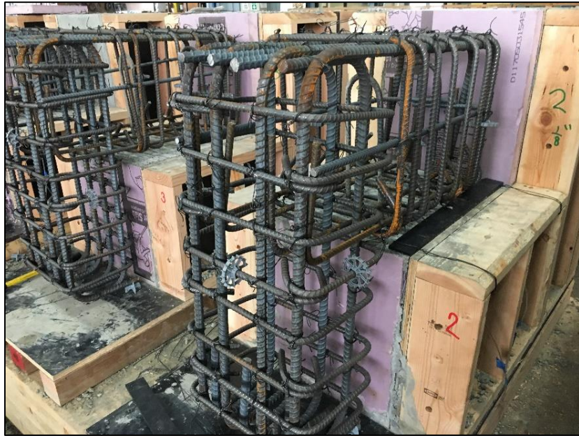
Figure 3.21: Top L-shaped cage placed on top of specimen.
