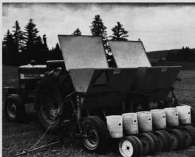
High-density planter with fertilizer banding attachment.
