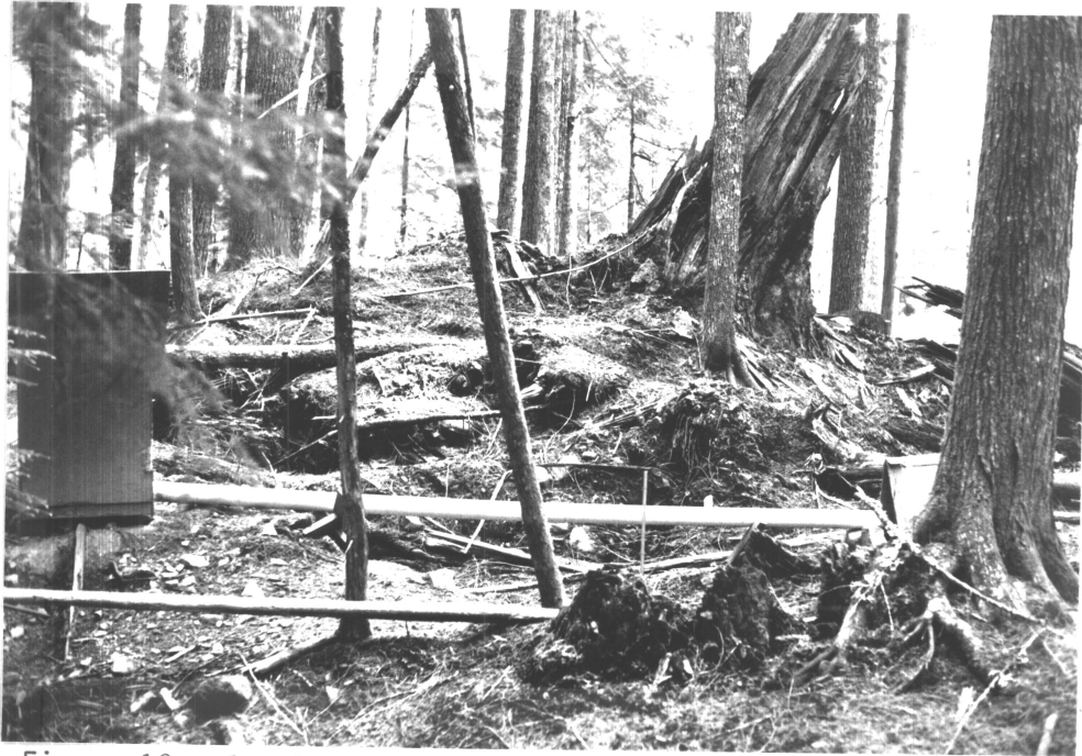
Figure 10. Crackmeter 2 across west boundary tension crack
