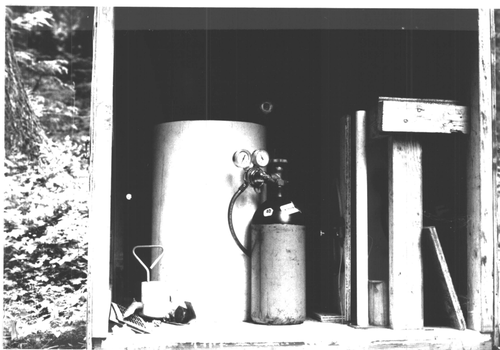
Figure 16. Instrumentation for recording groundwater levels.
