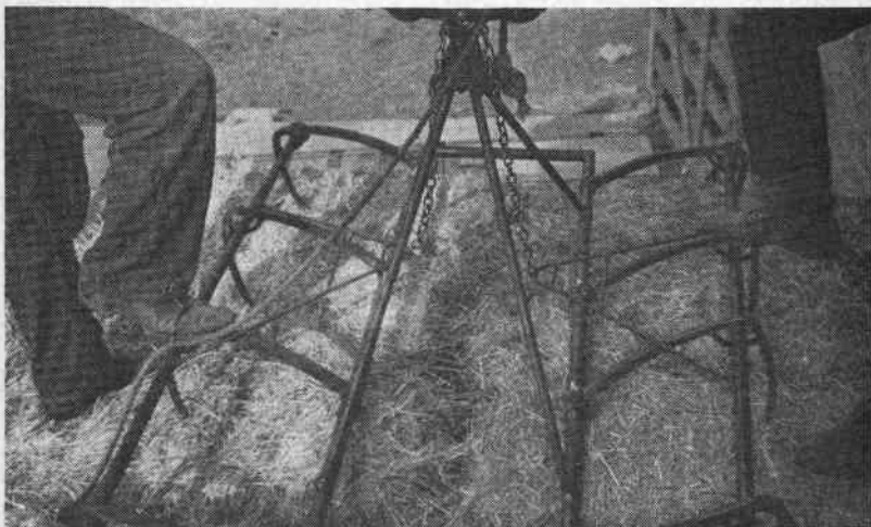
Figure 2. Inserting tines in bales. This can be accomplished rapidly by stepping on each tine.
