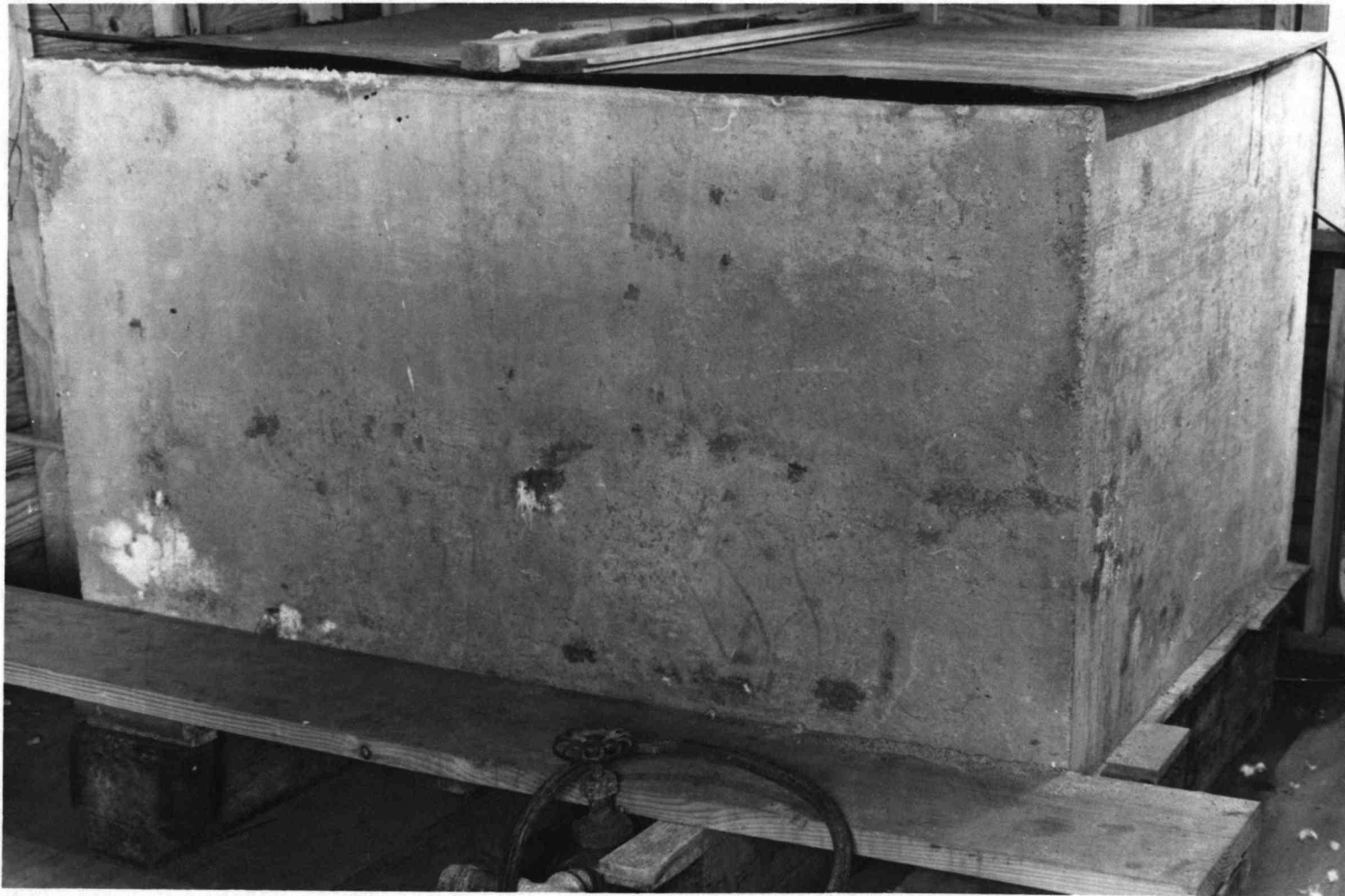
Figure 4 Temperature Controlled Concrete Tank
