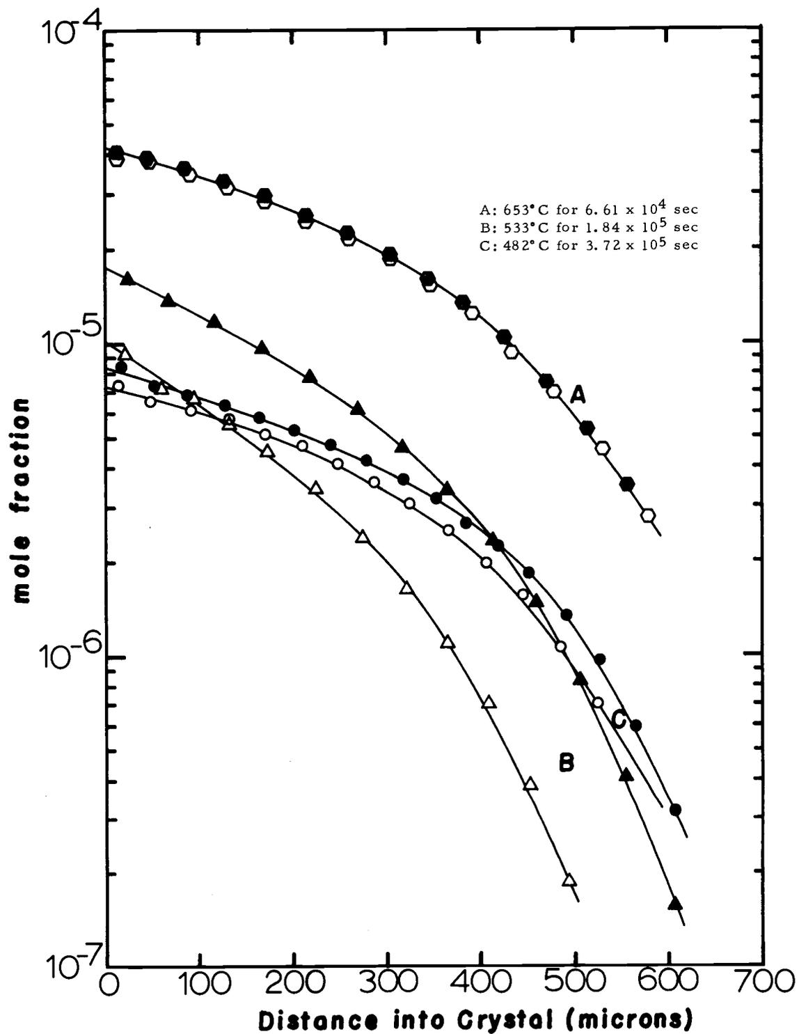
Figure 4. 6. Mole fraction of manganese as a function of distance into potassium chloride for various times and temperatures.
