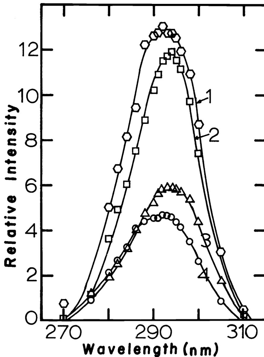
Figure 5.3. Reflectance spectra as a function of wavelength for various activator concentrations. 1:  $x_a = 1.5 \times 10^{-4}$ ; 2:  $x_a = 1.66 \times 10^{-4}$ ; 3:  $x_a = 5.8 \times 10^{-4}$ ; 4:  $x_a = 2.7 \times 10^{-5}$ .
