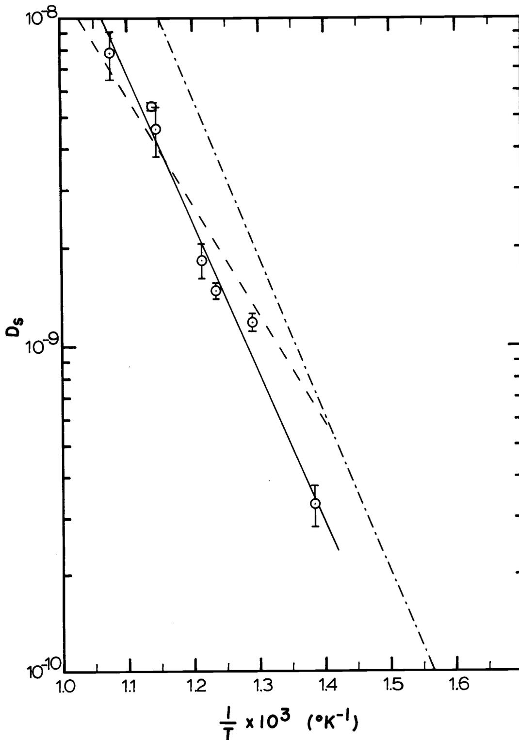
Figure 4. 3. Saturation diffusion coefficient for diffusion of manganese into sodium chloride as a function of reciprocal temperature ( $^{\circ}\text{K}^{-1}$ ). Solid line is from least squares fit to the data of this work, dashed line is that reported by Lure *et al.* and the dotted and dashed line is that reported by Stewart and Reed.
