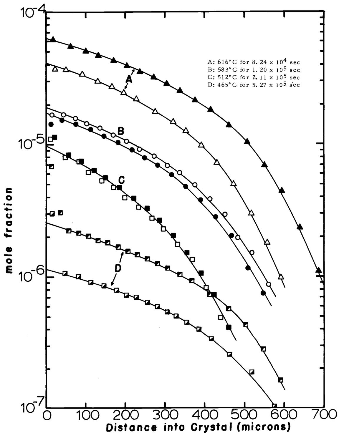
Figure 4. 5. Mole fraction of manganese as a function of distance into potassium chloride crystal for various times and temperatures.
