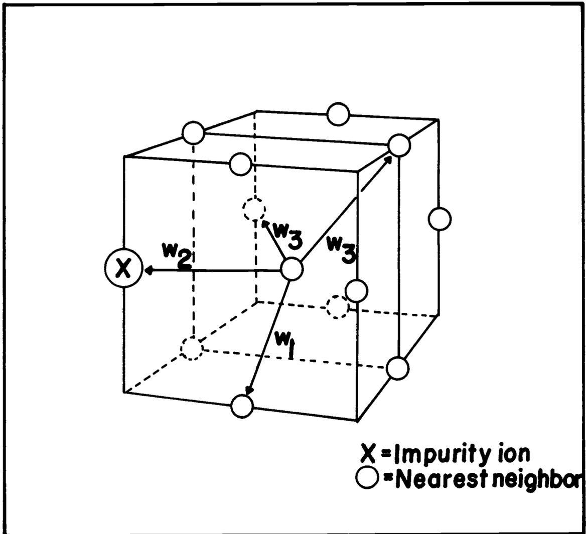
Figure 2.1 Diagram describing notation of jump probabilities.
