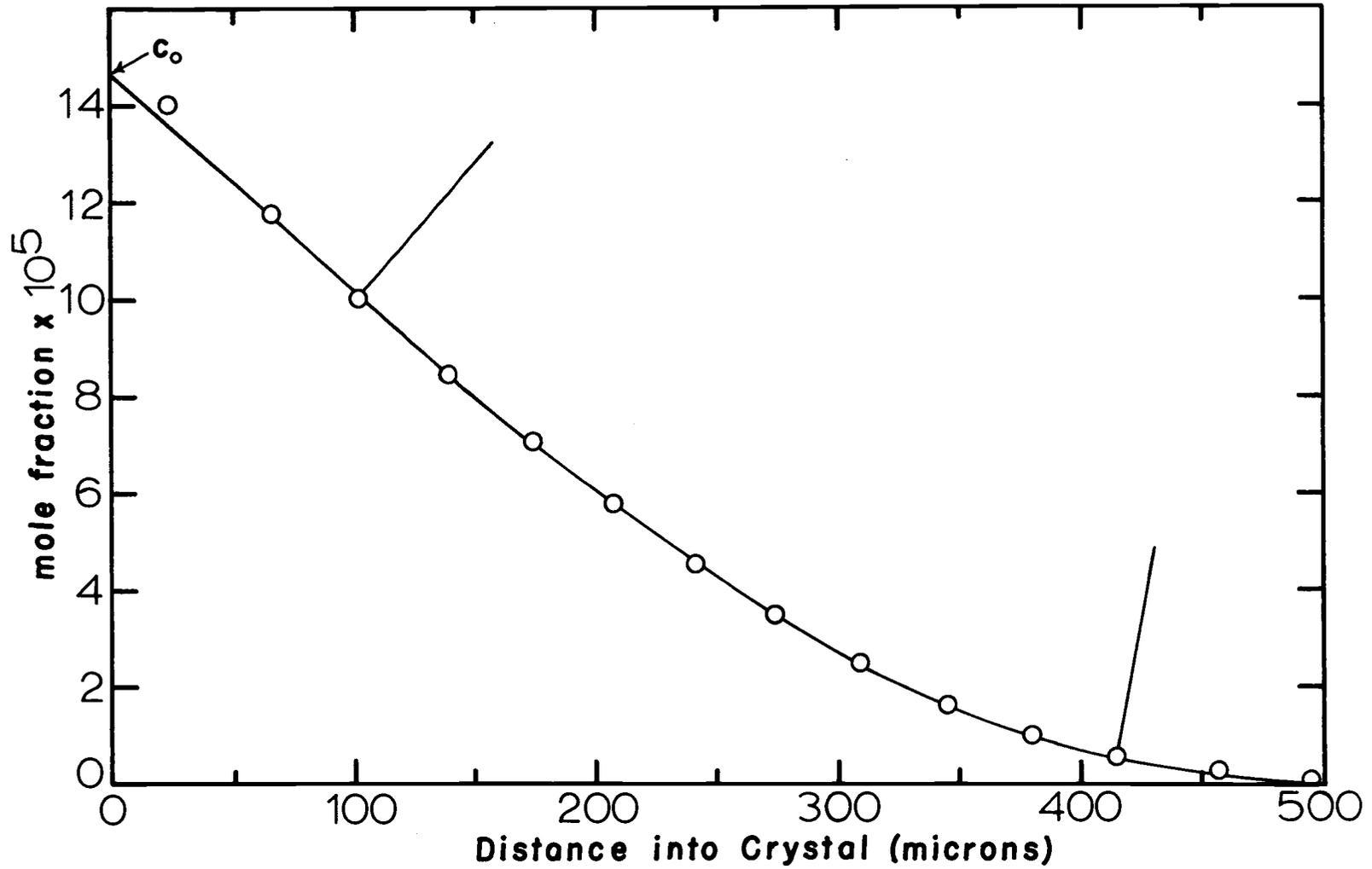
Figure 3. 1. Concentration of manganese as a function of distance into the crystal for a typical diffusion in sodium chloride. The lines at points 3 and 12 are perpendicular to the curve at that point and allow a measure of  $dc/dx$ .
