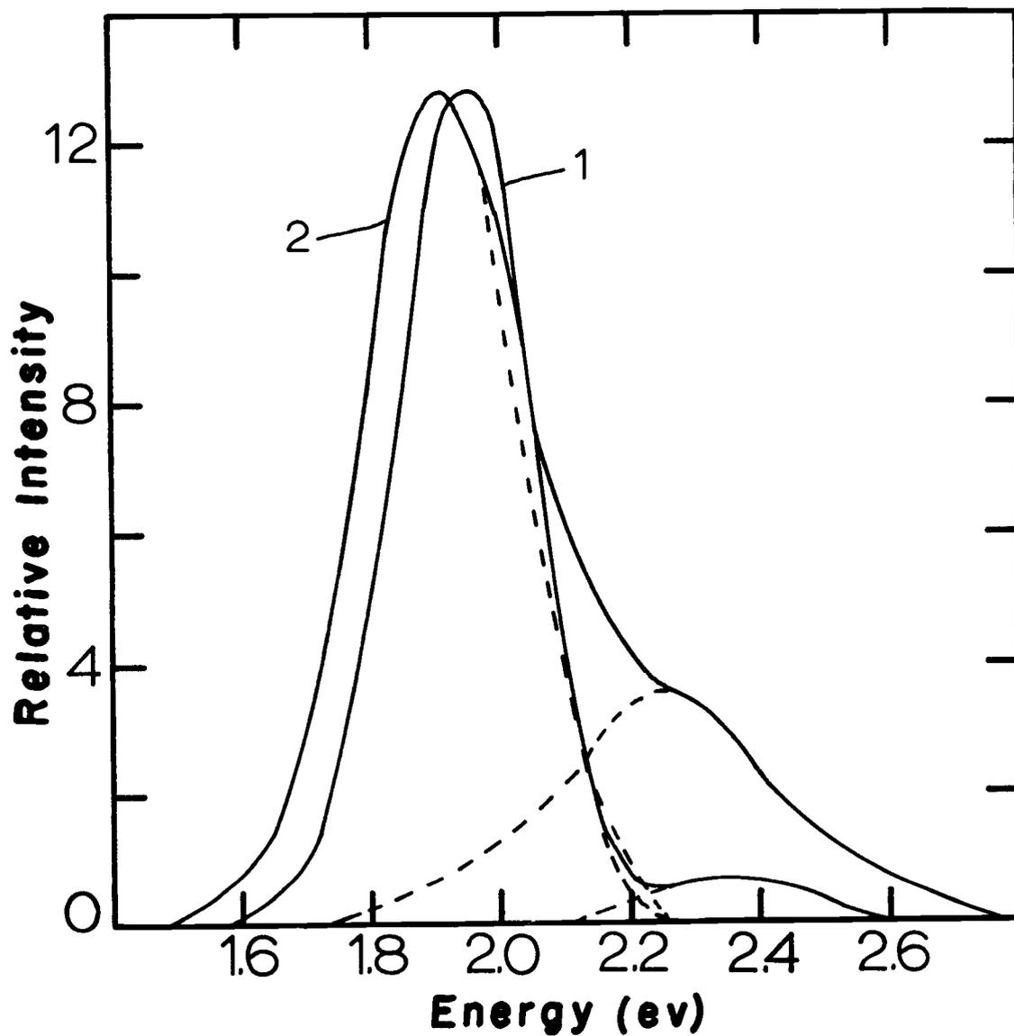
Figure 4.15. Growth of side band as a function of heat treatment for NaCl:Pb:Mn. Spectrum 1 is the sample quenched in liquid nitrogen after heating at 600°C for 15 minutes. Spectrum 2 is the same sample annealed to room temperature. Both curves normalized to the same main peak heights. Both curves obtained at  $90 \pm 3^\circ\text{K}$ .
