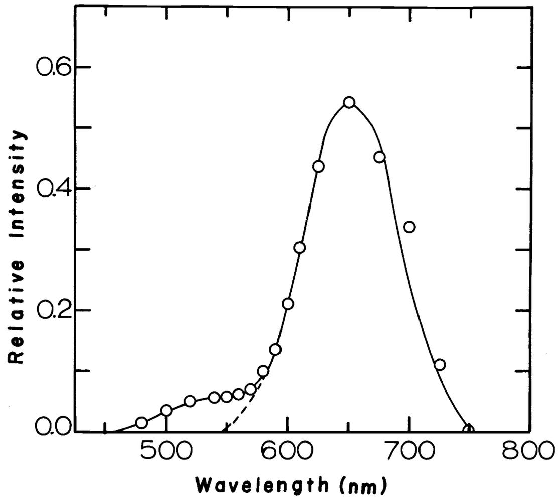
Figure 3. 3. Relative emission intensity as a function of wavelength. The area to the low wavelength side of the dotted line near 550 nm was omitted when measuring the area under the emission band. The area under the emission band is the area used in the numerator of equation (3. 17).
