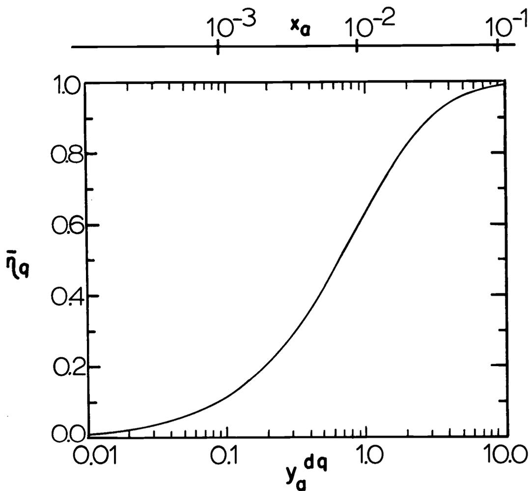
Figure 2.2 Quantum efficiency as a function of reduced activator concentration for dq transfer. The values of mole fraction of activator,  $x_a$ , are those estimated by Dexter.
