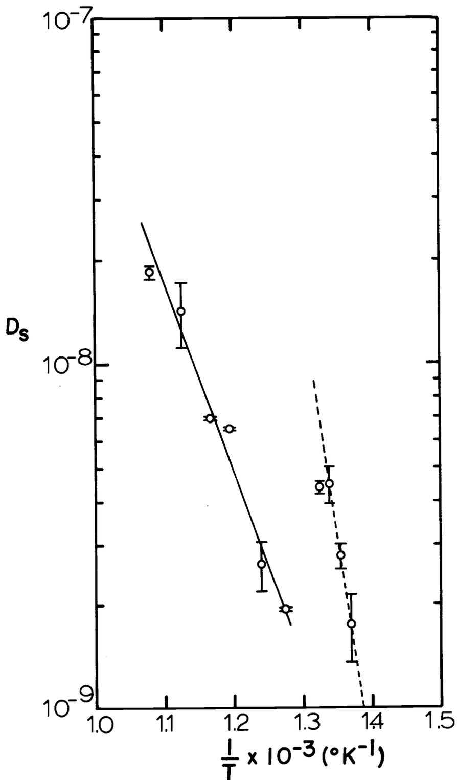
Figure 4.8. Saturation diffusion coefficient for diffusion of manganese into potassium chloride as a function of reciprocal temperature ( $^{\circ}\text{K}^{-1}$ ). Solid line at higher temperature is from least squares fit to the data along that line. Dashed line at lower temperatures is from least squares fit to the 3 points along it.
