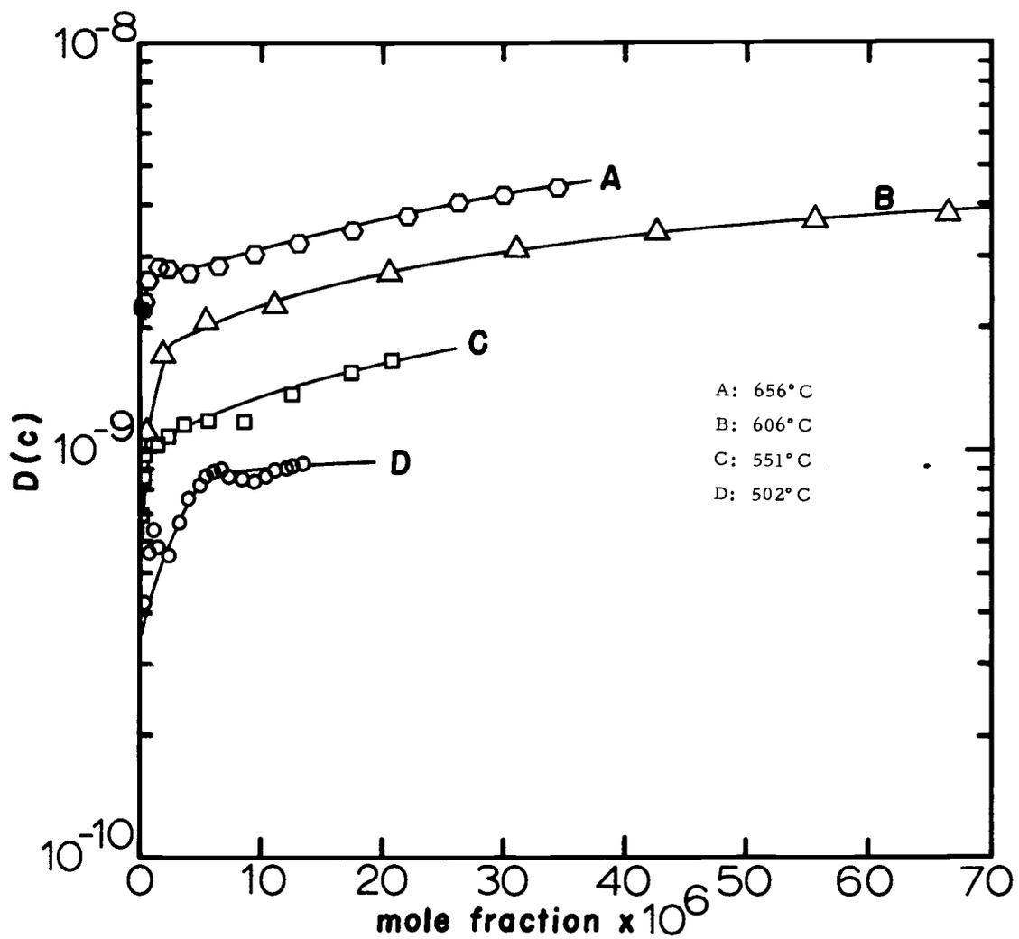
Figure 3. 2.  $D(c)$  as a function of concentration of manganese in NaCl for four experiments at different temperatures.
