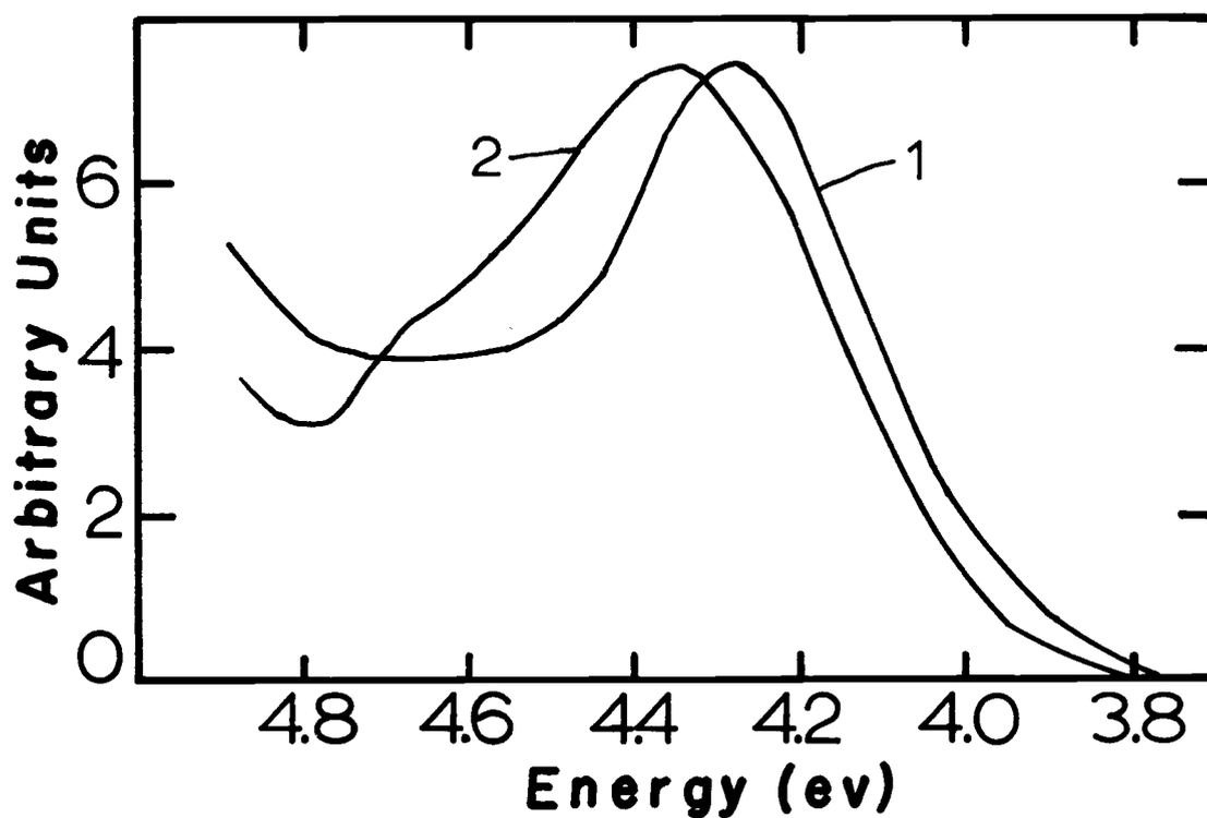
Figure 4.16. Excitation spectra for an annealed sample of NaCl:Pb:Mn. Spectrum 1 is the excitation curve for 2.26 eV emission. Spectrum 2 is the excitation curve for 1.92 eV emission. Both curves obtained at  $90 \pm 3^\circ\text{K}$ .
