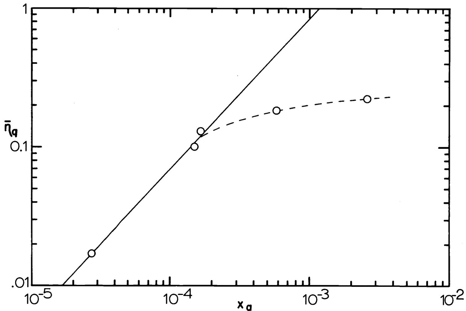
Figure 4.17. Average quantum efficiency,  $\bar{\eta}_q$ , as a function of  $x_a$  for the NaCl:Pb:Mn phosphor. The slope of the solid line is approximately one indicating linear dependence of the quantum efficiency on mole fraction of manganese in this region. Dashed line indicates the deviation from linearity as the concentration of manganese is increased. All quantum efficiency measurements made at  $90 \pm 3^\circ \text{K}$ .
