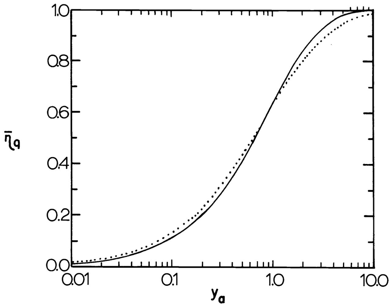
Figure 2. 3. Quantum efficiency as a function of reduced activator concentration for dd transfer (dotted line) and for qq transfer (solid line).
