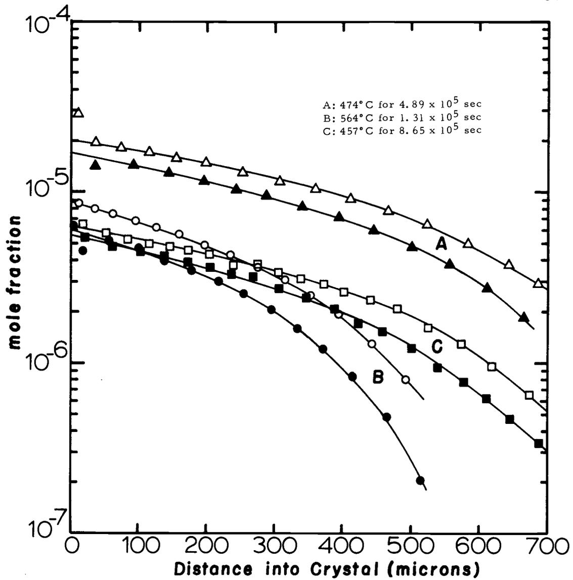
Figure 4.7. Mole fraction of manganese as a function of distance into potassium chloride for various times and temperatures.
