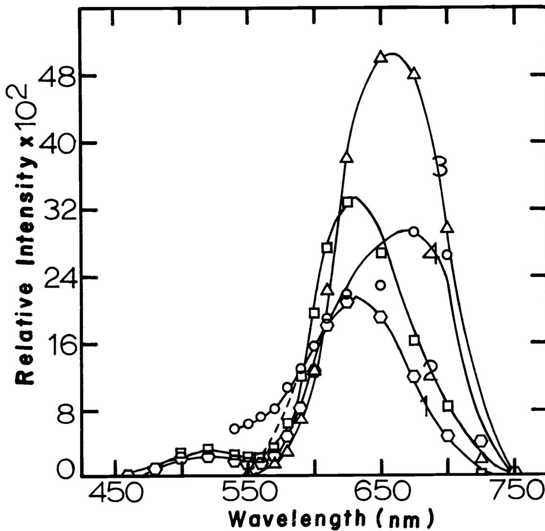
Figure 5.4. Emission spectrum as a function of wavelength for various activator concentrations. 1:  $x_a = 1.5 \times 10^{-4}$ ; 2:  $x_a = 1.66 \times 10^{-4}$ ; 3:  $x_a = 5.8 \times 10^{-4}$ ; and 4:  $x_a = 2.7 \times 10^{-5}$  (intensity multiplied by 10 to fit on scale).
