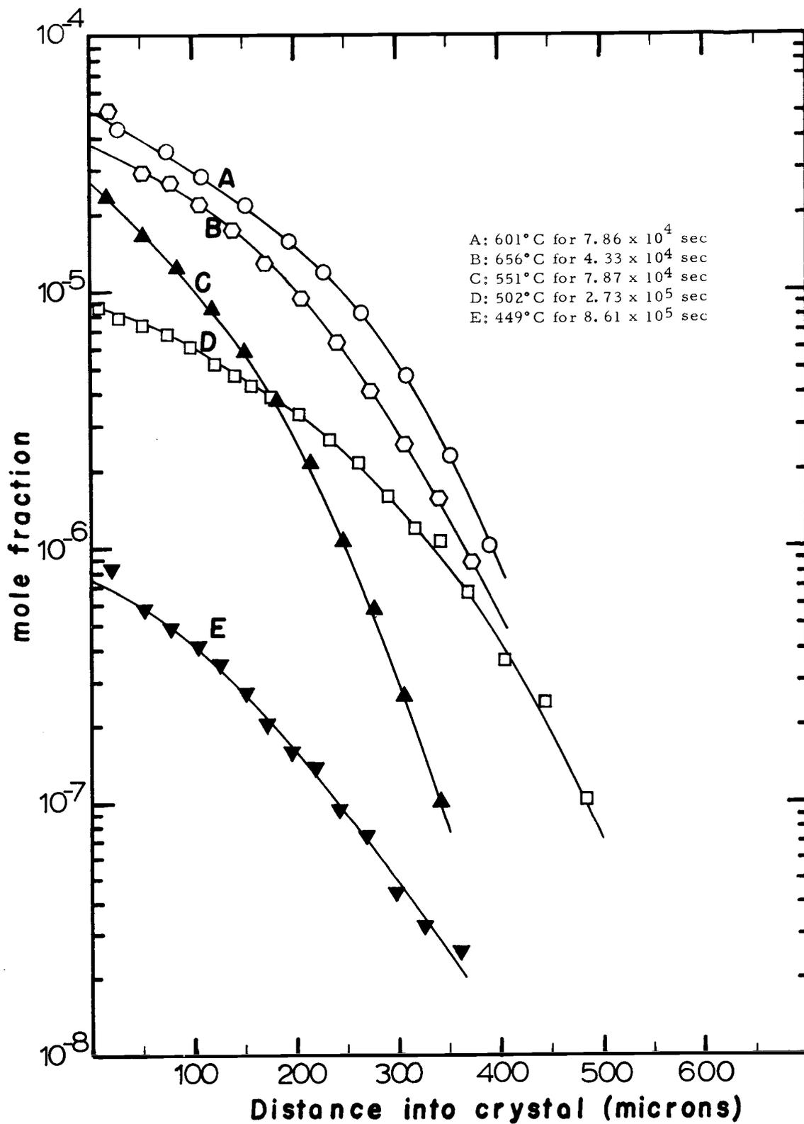
Figure 4. 1. Mole fraction of manganese as a function of distance into sodium chloride crystals for various times and temperature.
