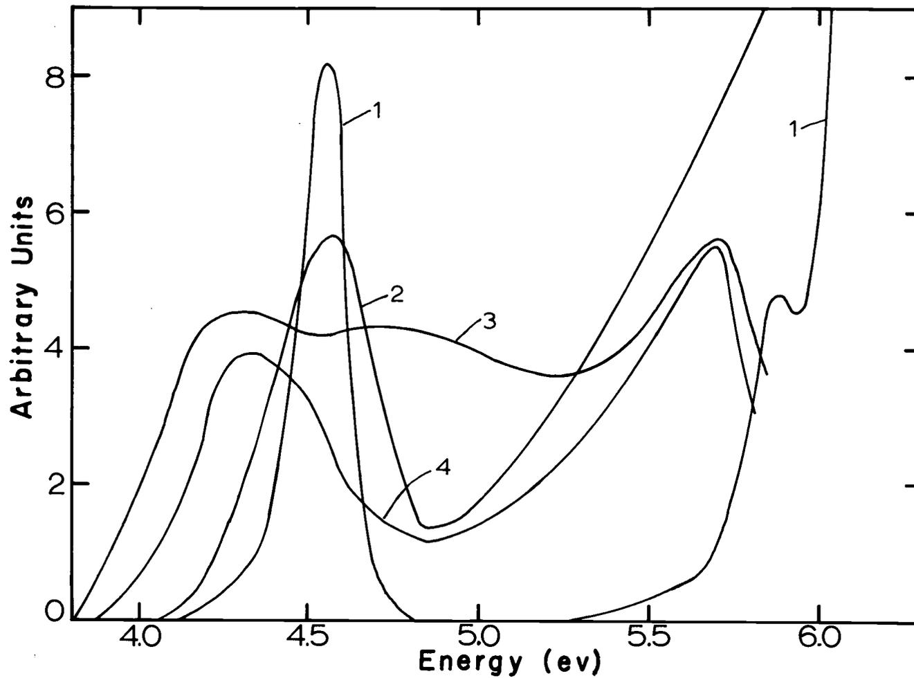
Figure 4.12. Absorption and excitation spectra for quenched and annealed samples of NaCl:Pb:Mn. Lines (1) absorption spectrum of quenched NaCl:Pb:Mn; (2) absorption spectrum of annealed NaCl:Pb:Mn; (3) excitation spectrum for emission of manganese for annealed NaCl:Pb:Mn and (4) excitation spectrum for manganese emission for quenched NaCl:Pb:Mn. All spectra at room temperature.
