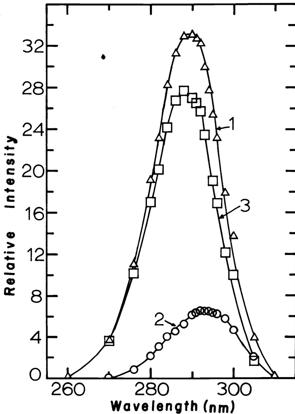
Figure 3.4. Relative intensity of reflected light as a function of wavelength. (1) reflection spectrum of "pure" NaCl; (2) reflection spectrum of doped NaCl, and (3) difference between 1 and 2. The area under 3 is the value for the denominator of equation (3.17).
