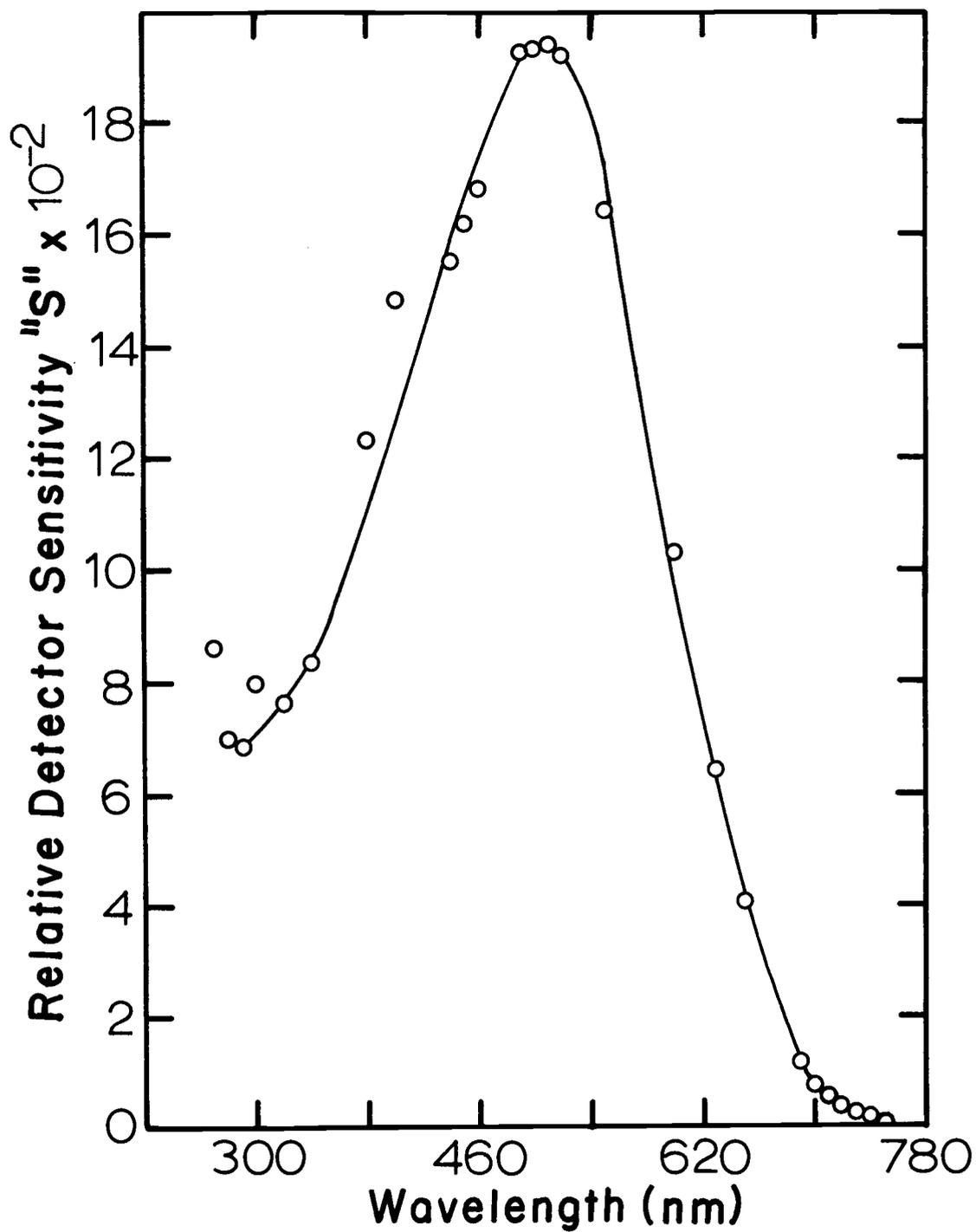
Figure 5. 1. Relative recorder deflection as a function of energy incident on the photomultiplier of the Perkin-Elmer 450 spectrophotometer.
