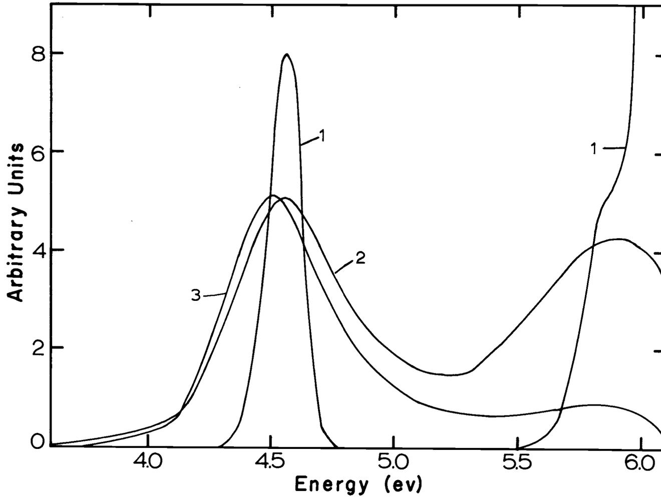
Figure 4.13. Absorption and emission spectra for quenched and annealed KCl:Pb:Mn. Lines (1) absorption spectra of quenched and annealed KCl:Pb:Mn; (2) excitation spectrum for manganese emission for quenched KCl:Pb:Mn and (3) excitation spectrum for manganese emission for annealed KCl:Pb:Mn phosphor. All spectra at room temperature.
