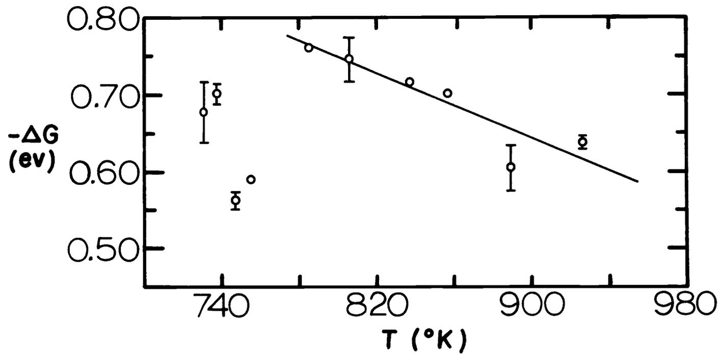
Figure 4. 9. Free energy of association as a function of temperature for manganese in potassium chloride. The straight line is a least squares fit to the data along that line. Those points that have no error limits signify experiments that showed identical  $-\Delta G$ 's for both crystals at that temperature.
