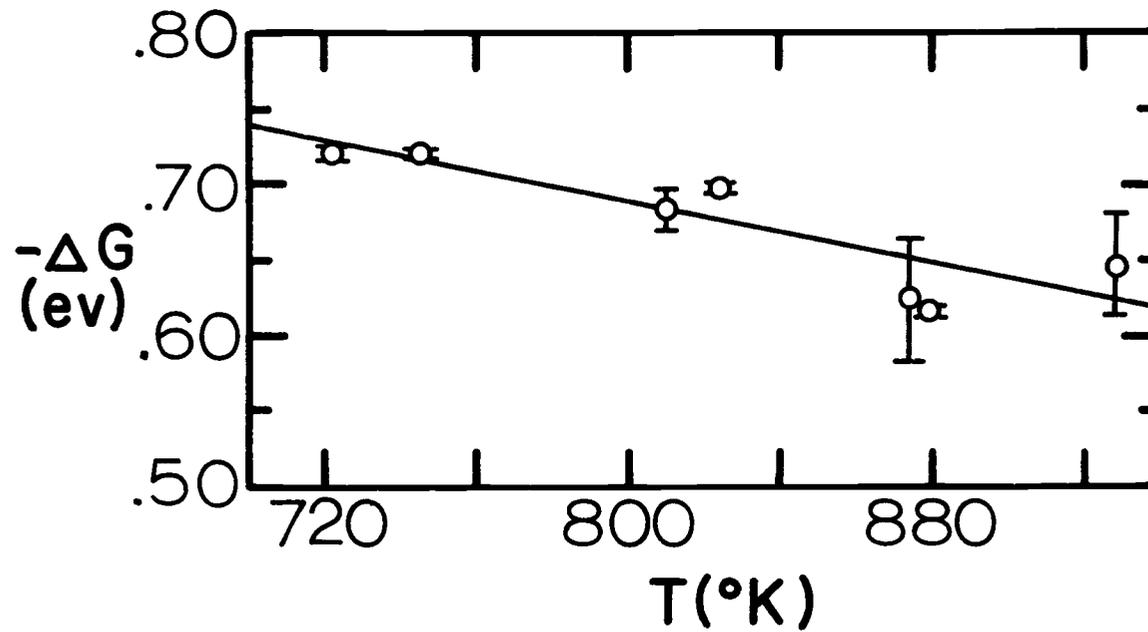
Figure 4.4. Free energy of association as a function of temperature for manganese in sodium chloride. The straight line is a least squares fit to the data points. The entropy of association is found from the slope of the straight line, i. e.  $\Delta S = \partial(-\Delta G)/\partial(T)$ .
