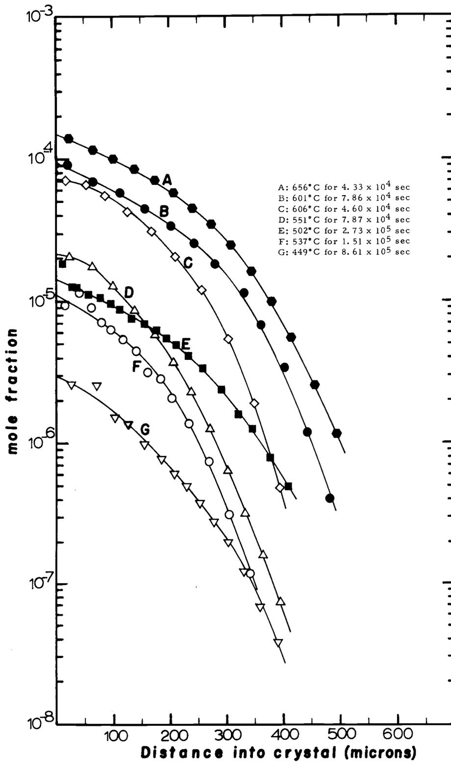
Figure 4. 2. Mole fraction of manganese as a function of distance into sodium chloride crystal for various times and temperatures.
