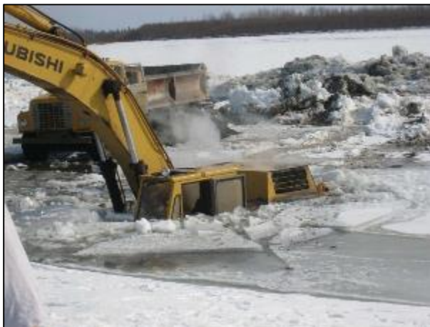
Figure 8 – Local Galena excavator that broke through the Yukon River ice (Doig and Olsen 2013).
