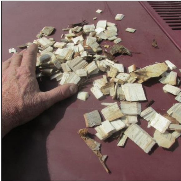
Figure 22 – Sample of chips processed through the Bandit M1400.
