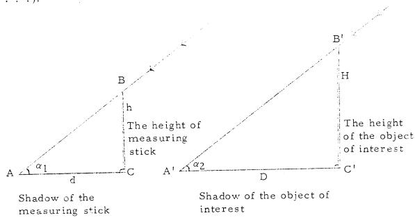
Notice: In case of using the sunbeam, the measurements must be taken at nearly the same time, because the angle of its incident may change.
