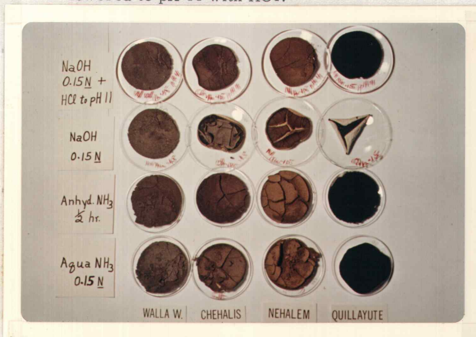
Figure 5. Air-dried residues of soils extracted with 0.015 \underline{N} \text{NH}_4\text{OH} , 0.15 \underline{N} \text{NH}_4\text{OH} , and 0.15 \underline{N} \text{NaOH} with pH lowered to pH 11 with \text{HCl} .
