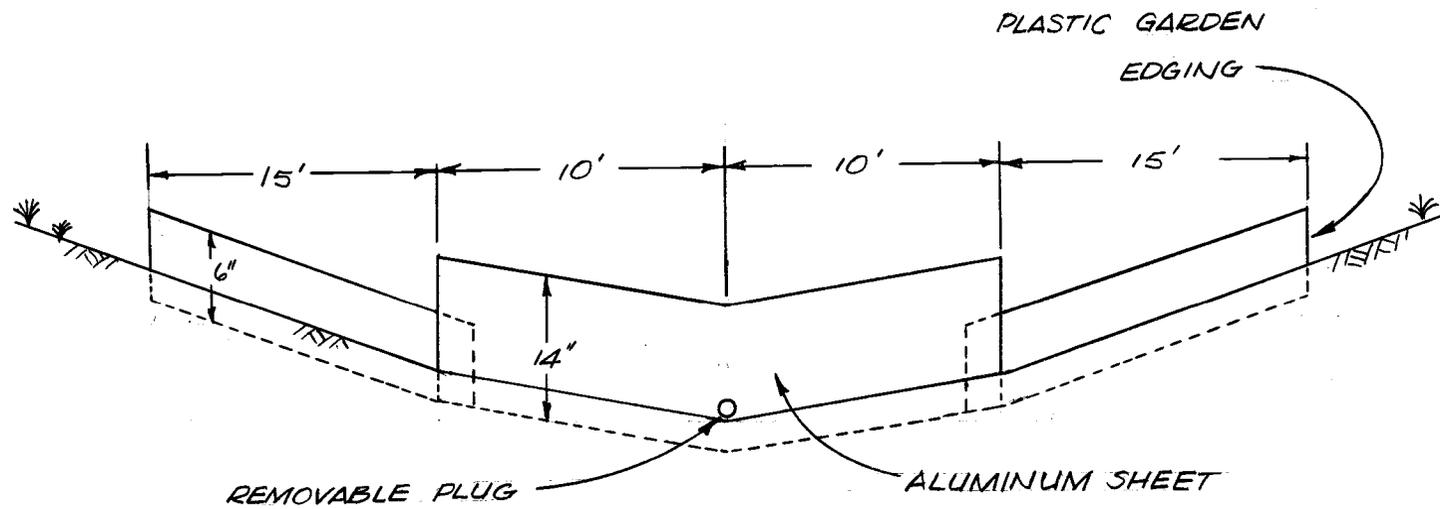
Figure 4. Typical runoff collection dam.
