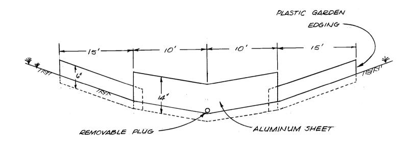
Figure 4. Typical runoff collection dam.
