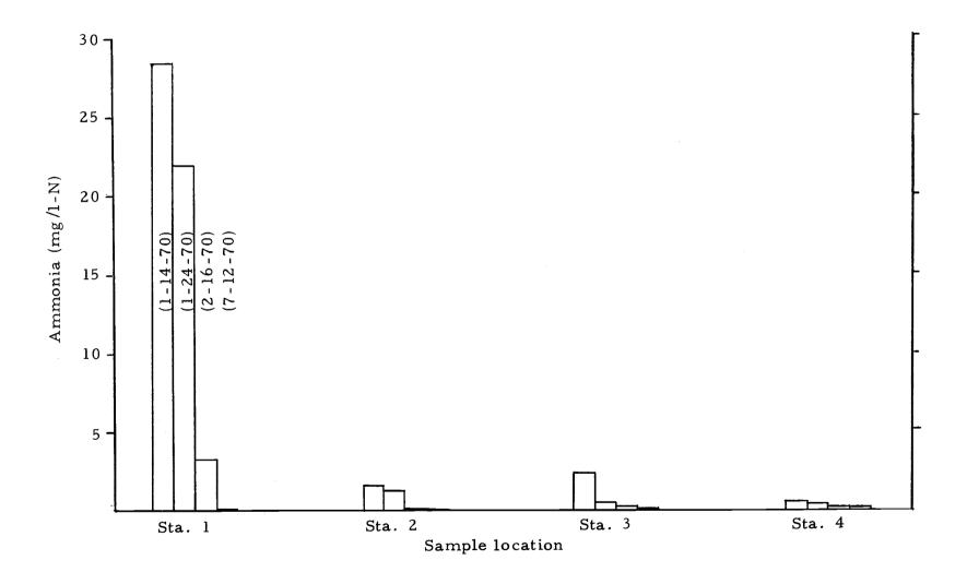
Figure 5. Ammonia-N versus sample station.
