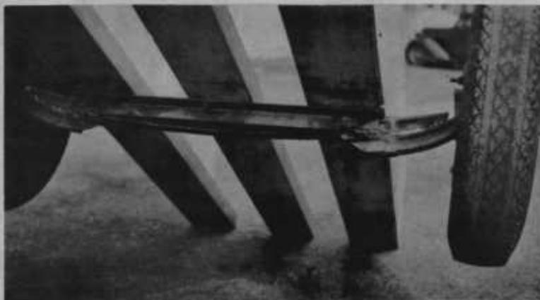
Figure 3. Axle with main floor stringers and angle irons.
