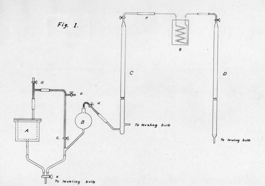
used for forcing mercury into either A or B.
