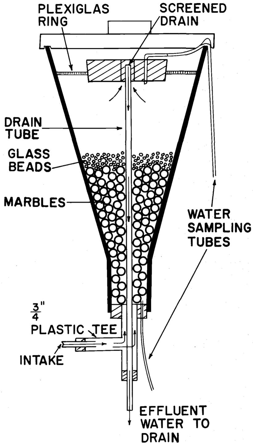
Figure 2. Cut-away view of the respirometer-rearing chamber used for holding steelhead trout embryos and alevins at constant levels of dissolved oxygen and NaPCP.
