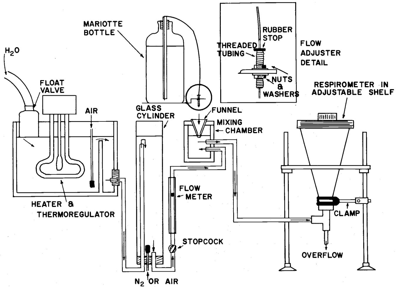
Figure 3. Diagram of the apparatus used in studies of the effect of dissolved oxygen concentration on the toxicity of NaPCP.
