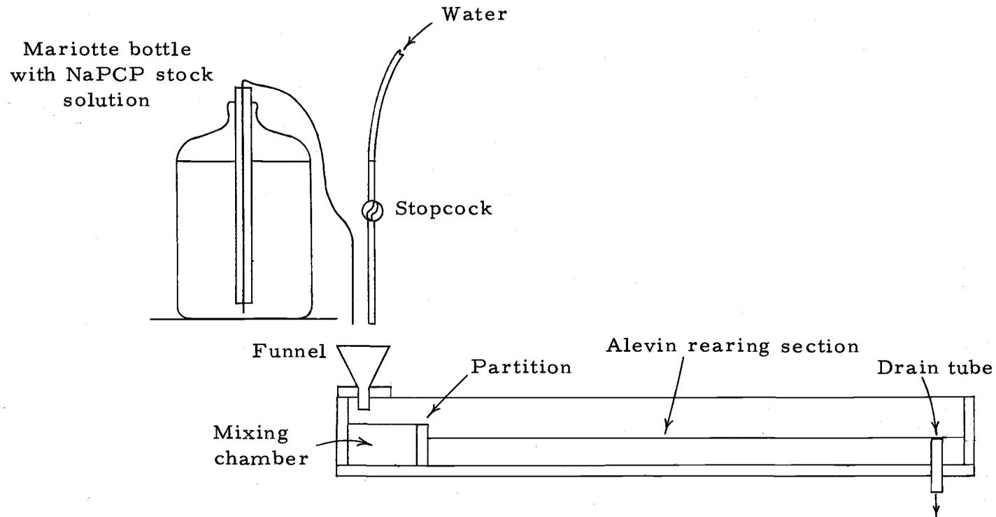
Figure 1. Side view of one of the troughs used for rearing alevins in a constantly renewed solution of NaPCP.
