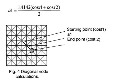
But when determining the cumulative cost for diagonal movement, the following formula must be used:
