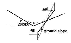
Fig. 23 Vertical effect on earthwork calculation.
