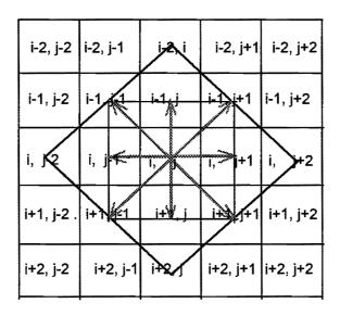
Fig.15 Slope and earth work calculation. Earth work calculation Slope calculation
