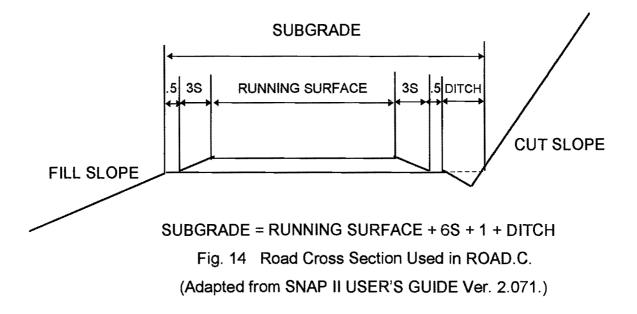
Road sections are assumed to be either balanced or full bench. If the slope is greater than 60%, the full bench section will be used. As with SNAP,
