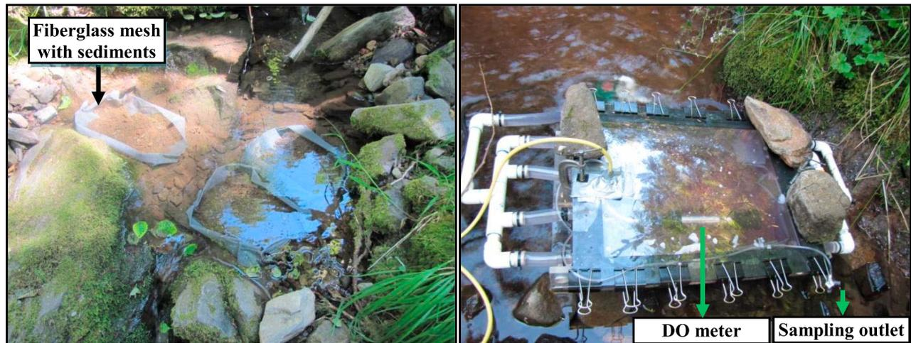
**Figure 3.** Respiration chamber experiments conducted at the H. J. Andrews Experimental Forest to test the correlation between  $\Delta Rru$  and  $\Delta DO$ : (left) fiberglass incubation meshes; (right) recirculating chamber with incubated sediments.
