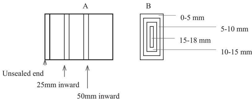
Figure 1. — Cutting patterns used to sample MC of Trex samples. A) Pattern used to cut 5-mm-thick slices from 100-mm-long samples; B) Pattern used to sample moisture gradients in Trex slices.
