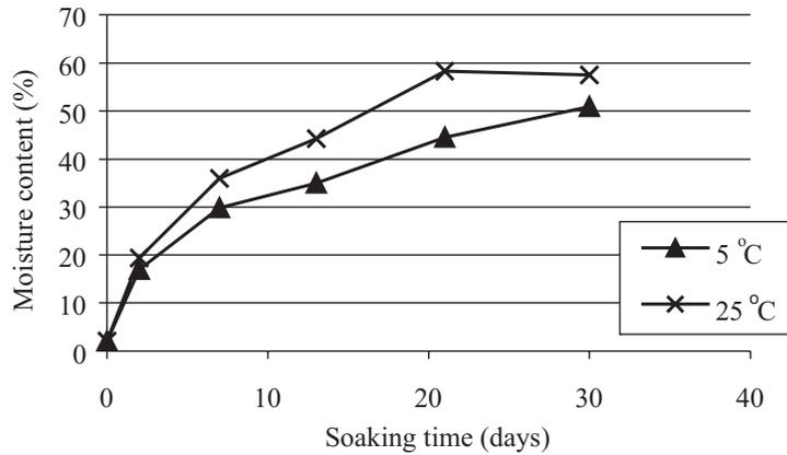
Figure 7. — Effect of water temperature on wood MC in the outer 5 mm of Trex samples immersed for 30 days at 5°C or 25°C.
