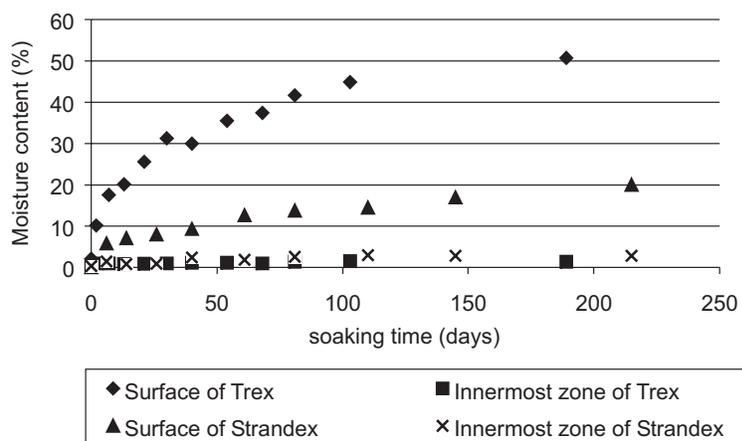
Figure 3. — Wood MC in surface (0 to 5 mm) and inner zones (15 to 18 mm and 10 to 12 mm) of Trex and Strandex samples immersed in water for up to 215 days.
