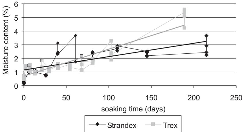
Figure 4. — Wood MCs of Trex and Strandex samples cut 5 to 10 mm inward from the surfaces of cross sections cut 25 mm in from the exposed cross section.
