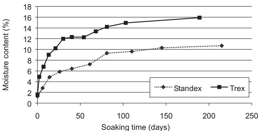
Figure 2. — Overall wood MC of 100-mm-long Trex and Strandex samples soaked in water at 5°C for up to 215 days.
