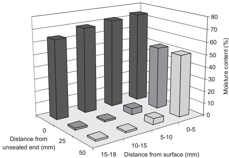
Figure 5. — Wood MC variation of Trex immersed in water for 190 days at 5°C.
