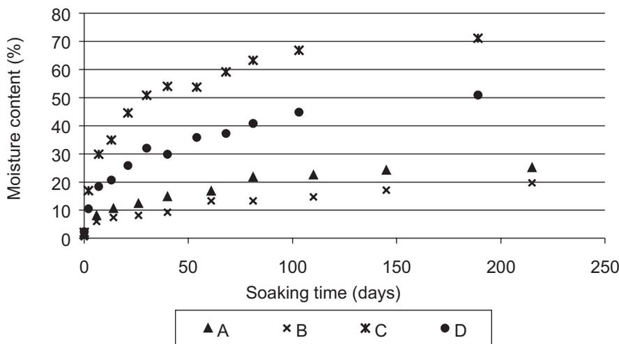
Figure 6. — Wood MC in the outer 5 mm of Strandex (A and B) or Trex (C and D) adjacent to the cut end (A and C) and 25 mm inward from that zone (B and D).
