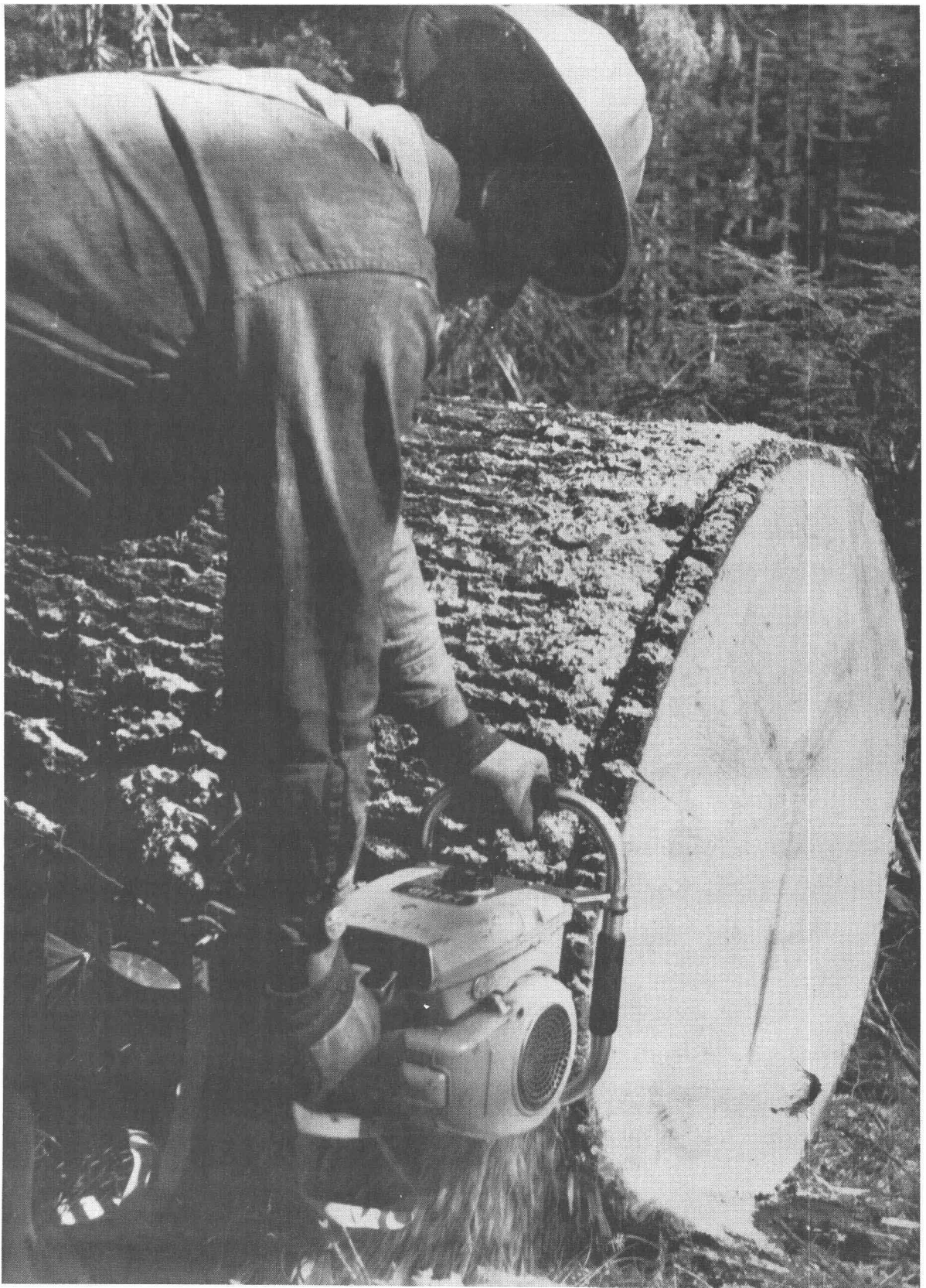
Figure 1.--Sawing sample disk from 40-inch Douglas-fir in northern California.
