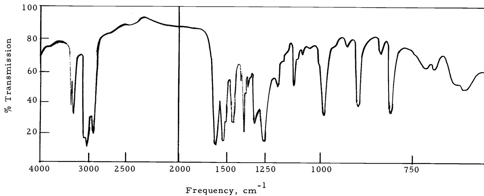
Figure 32. Infrared spectrum of 4-hydrazino-6-methoxy-5-nitropyrimidine.
