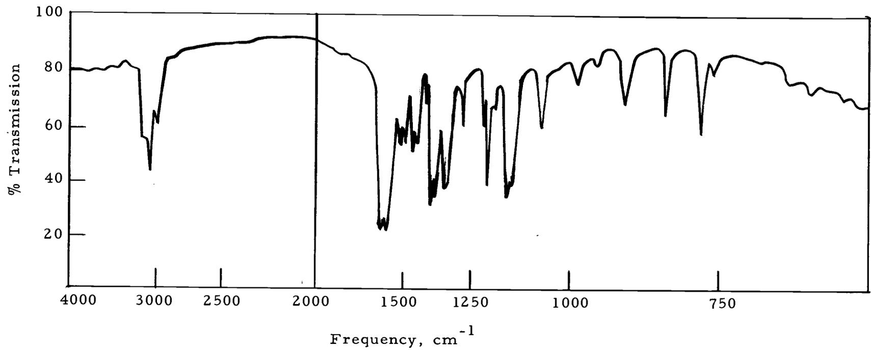
Figure 36. Infrared spectrum of 5-nitro-2,4,6-trimethoxypyrimidine.
