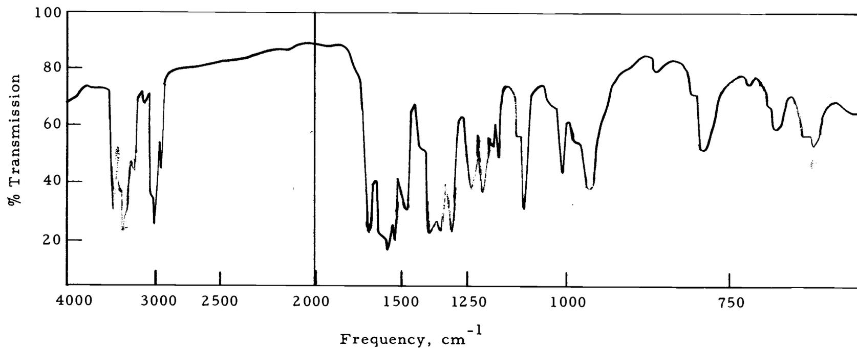
Figure 20. Infrared spectrum of dihydrazino-methoxy-5-nitropyrimidine.
