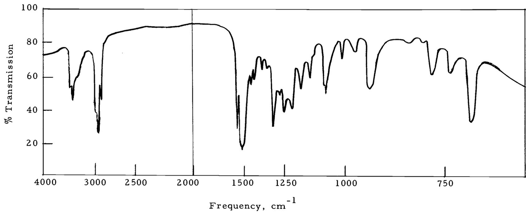
Figure 22. Infrared spectrum of 4,6-dihydrino-5-nitro-2-phenylpyrimidine.
