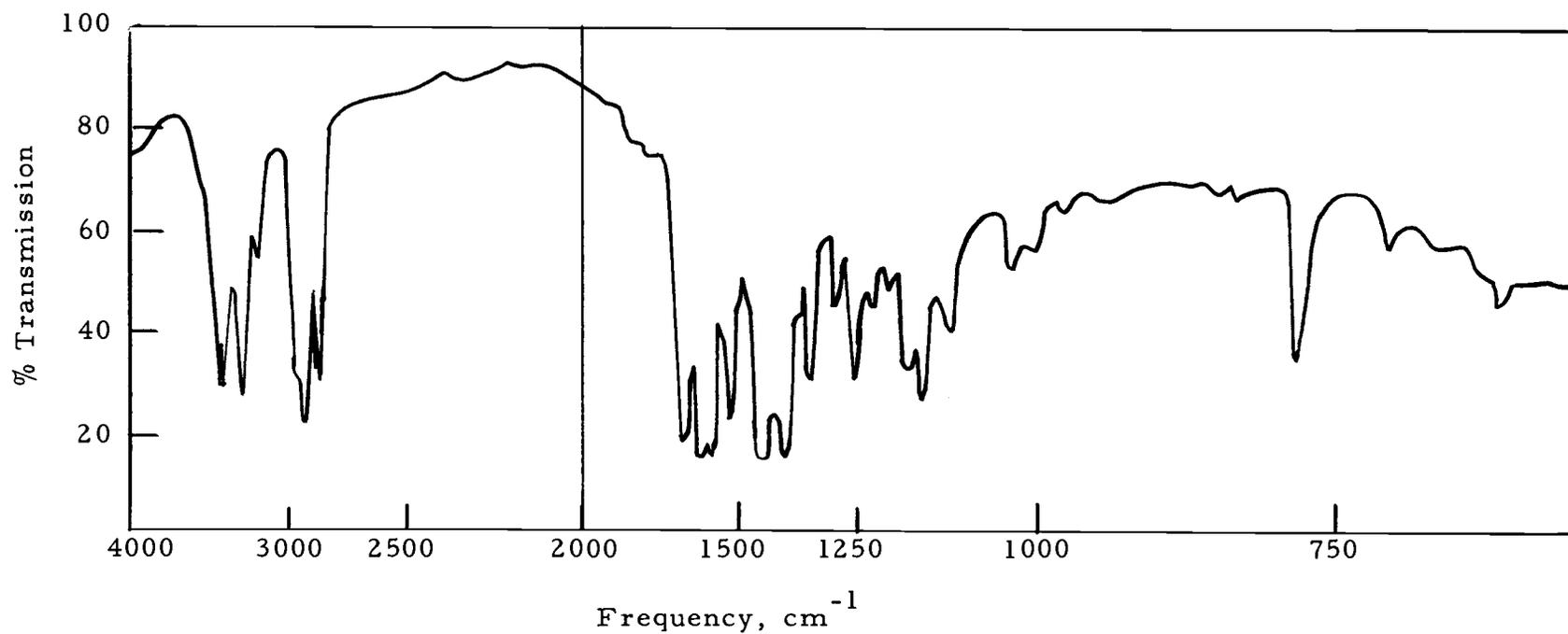
Figure 35. Infrared spectrum of 4-methylamino-6-(1-methylhydrazino)-5-nitropyrimidine.
