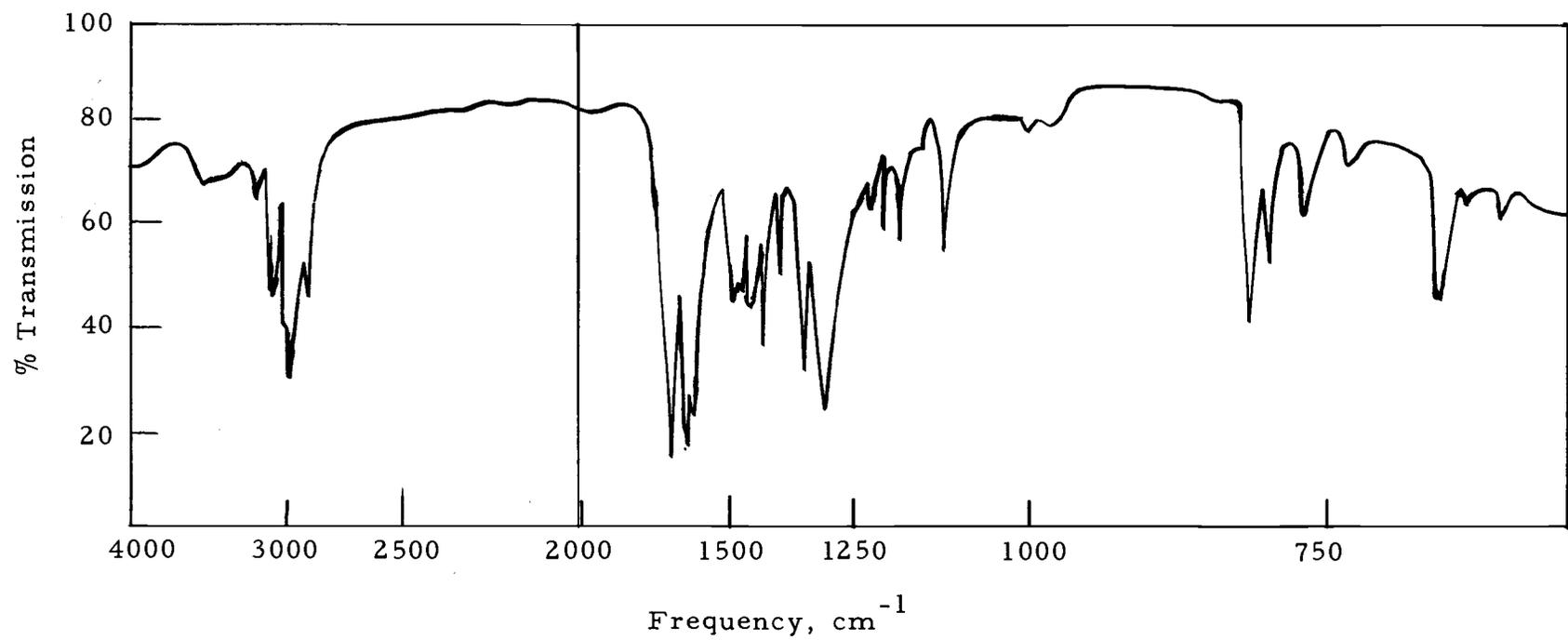
Figure 15. Infrared spectrum of N-methylpyridinium pyrimidinate salt (XXXII).
