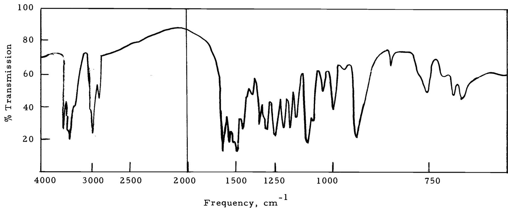
Figure 21. Infrared spectrum of 4,6-dihydrazino-2-methyl-5-nitropyrimidine.
