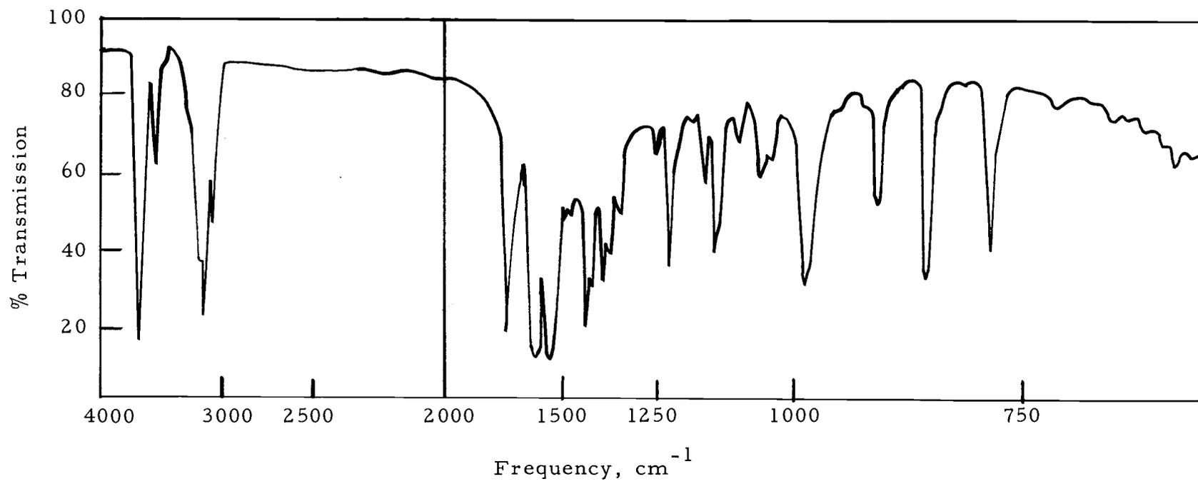
Figure 27. Infrared spectrum of 4,6-di-(1-methylhydrazino)-2-methyl-5-nitropyrimidine.
