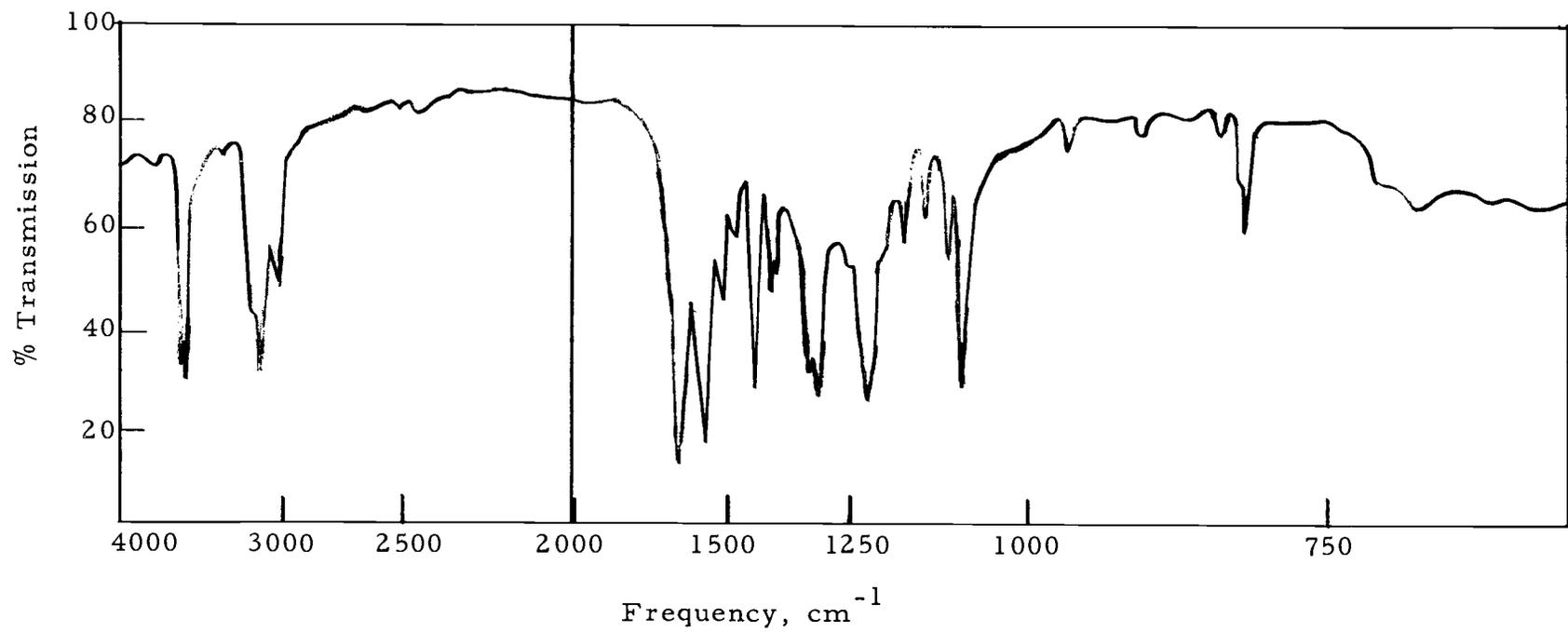
Figure 25. Infrared spectrum of 4-dimethylamino-6-(1-methylhydrazino)-5-nitropyrimidine.
