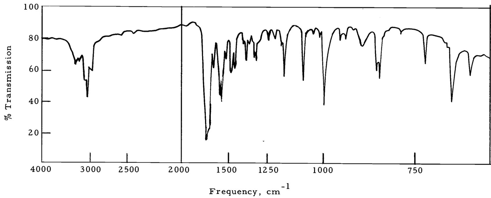
Figure 18. Infrared spectrum of 4-chloro-6-hydroxy-2-phenylpyrimidine.
