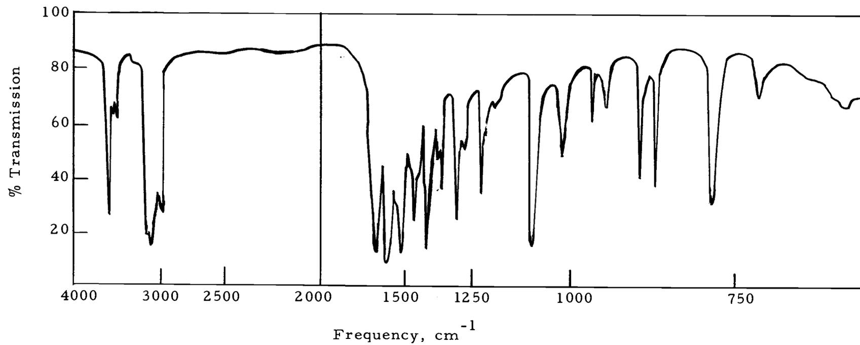
Figure 34. Infrared spectrum of 4-methoxy-6-(1-methylhydrazino)-5-nitropyrimidine.
