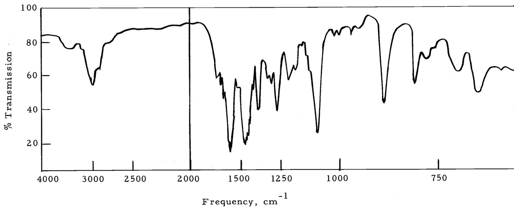
Figure 16. Infrared spectrum of residue from evaporation of XXXIV filtrate.
