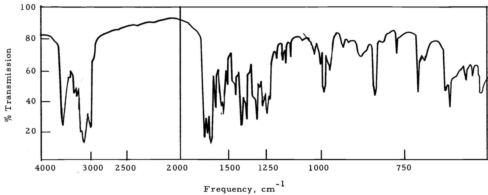
Figure 10. Infrared spectrum of acetylated 2Ph-K (nujol mull).
