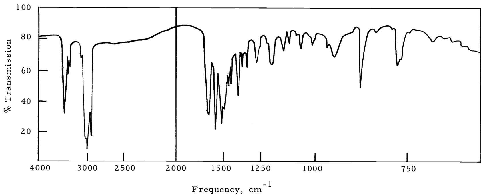
Figure 29. Infrared spectrum of 4,6-di-(1-methylhydrazino)-5-nitropyrimidine.
