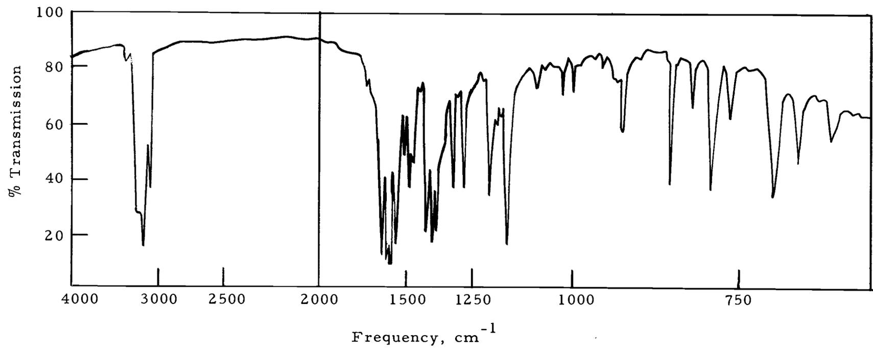
Figure 23. Infrared spectrum of 4,6-dimethoxy-5-nitro-2-phenylpyrimidine.
