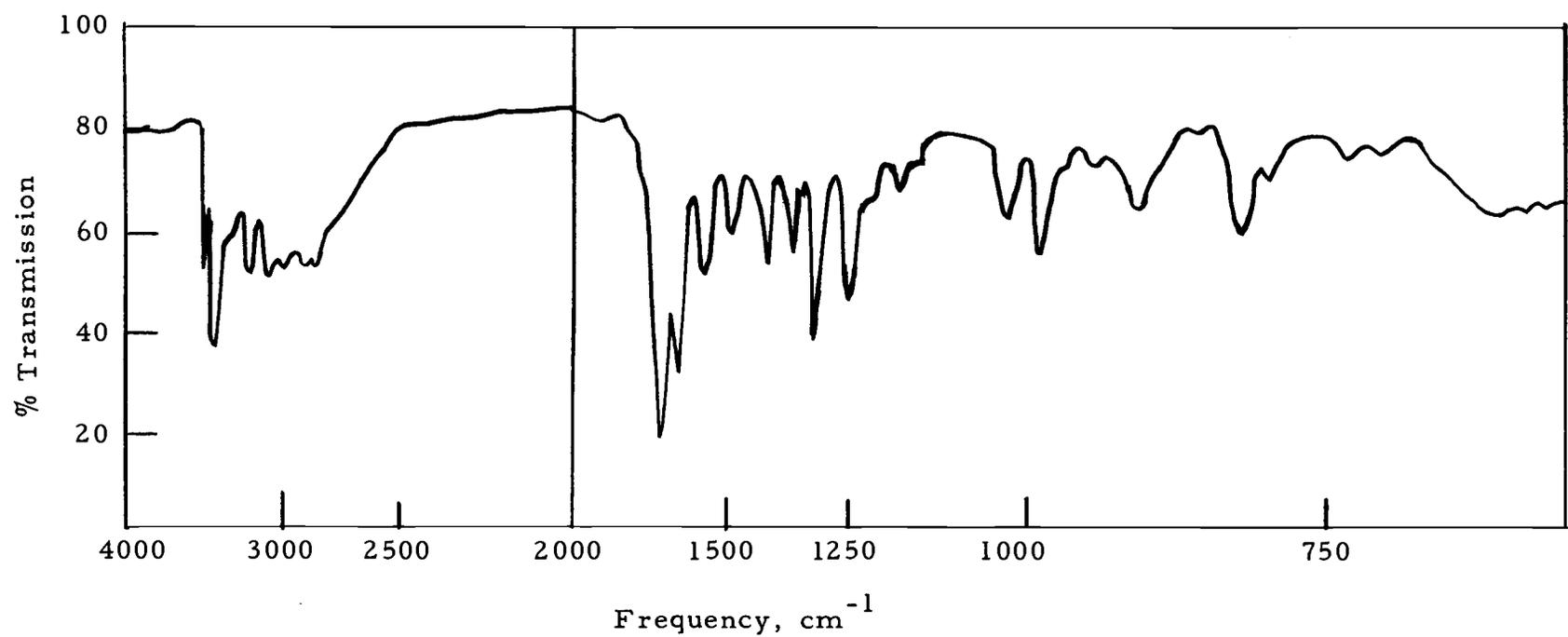
Figure 3. Infrared spectrum of 2H-K; composite of mulls in Kel-F-10 oil (4000-1300 cm<sup>-1</sup>) and nujol oil (1300-625 cm<sup>-1</sup>).
