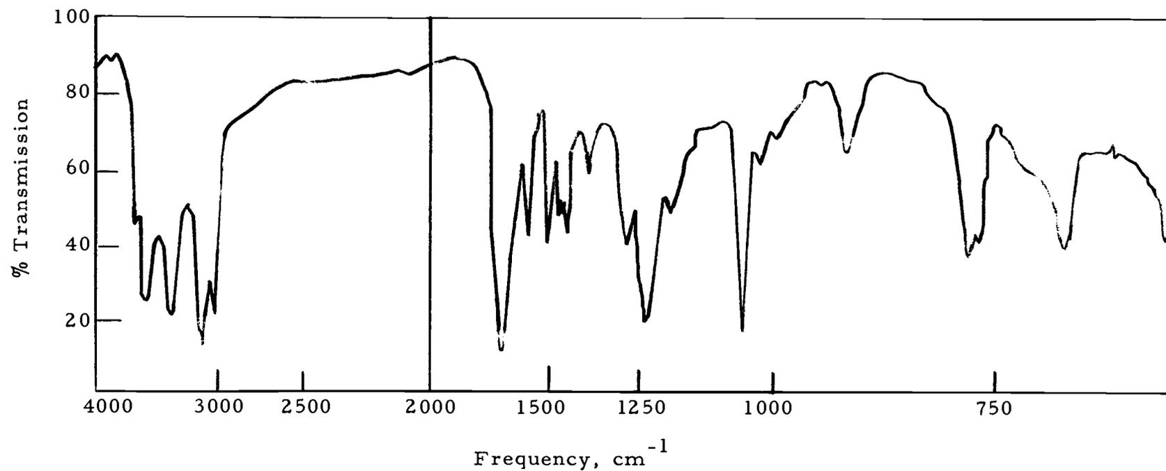
Figure 19. Infrared spectrum of 4,6-diamino-5-pyrimidyl hydrogen sulfate.
