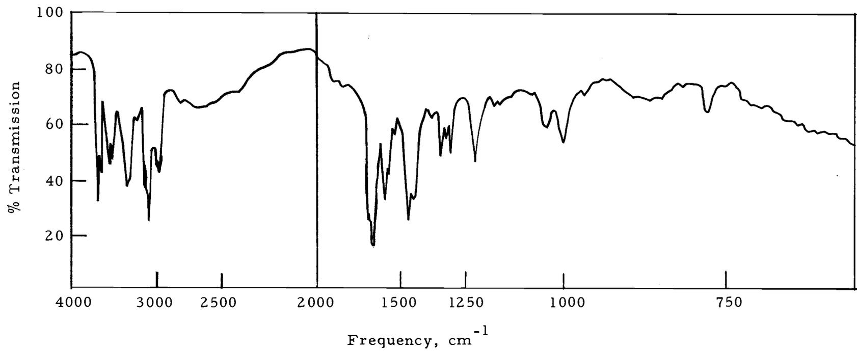
Figure 12. Infrared spectrum of 4,6-diamino-6-hydroxypyrimidine (nujol mull).
