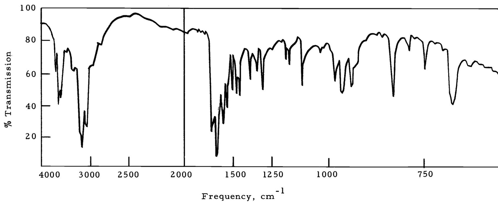
Figure 6. Infrared spectrum of 2Ph-K (nujol mull).
