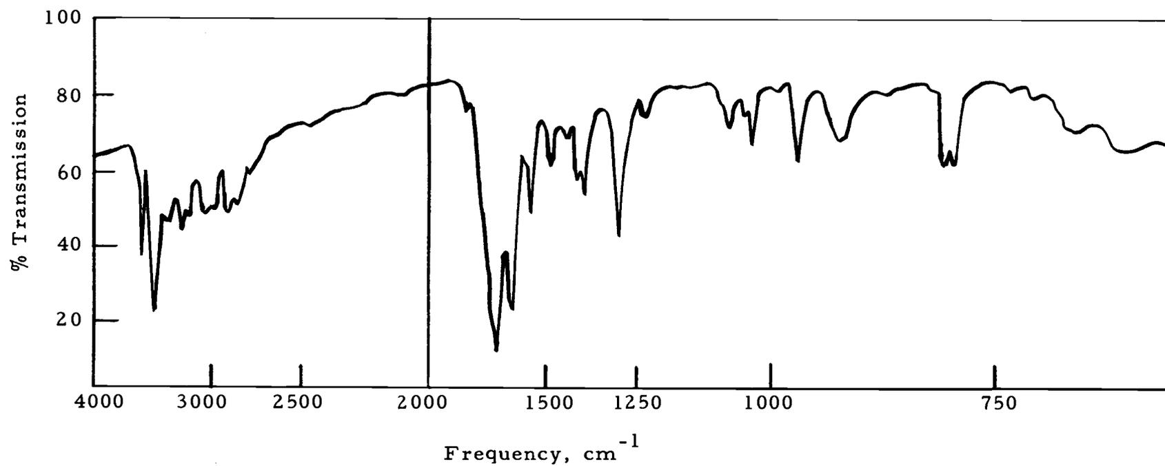
Figure 4. Infrared spectrum of 2Me-K; composite of mulls in Kel-F-10 oil (4000-1300 cm<sup>-1</sup>) and nujol oil (1300-625 cm<sup>-1</sup>).
