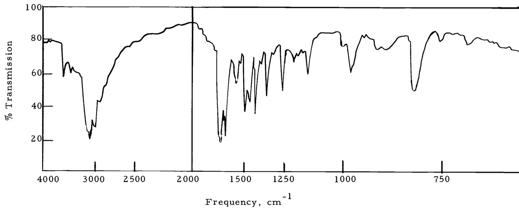
Figure 33. Infrared spectrum of 4-hydroxy-6-(1-methylhydrazino) pyrimidine.
