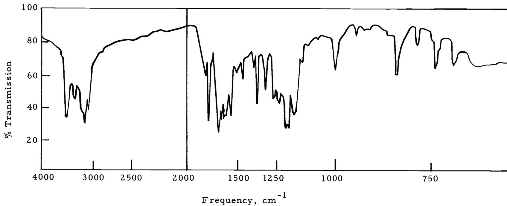
Figure 5. Infrared spectrum of residue from solution of 2H-K in trifluoroacetic acid.
