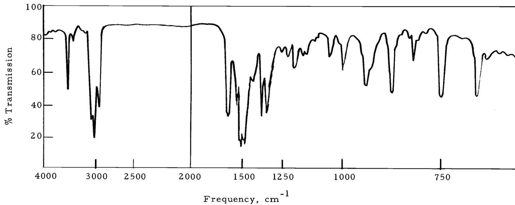
Figure 28. Infrared spectrum of 4,6-di-(1-methylhydrazino)-5-nitro-2-phenylpyrimidine.
