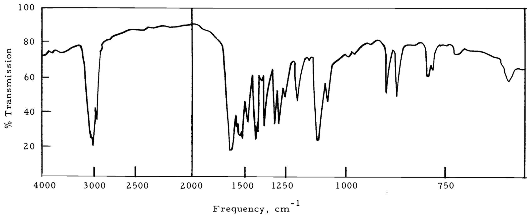
Figure 24. Infrared spectrum of 4-dimethylamino-6-methoxy-5-nitropyrimidine.
