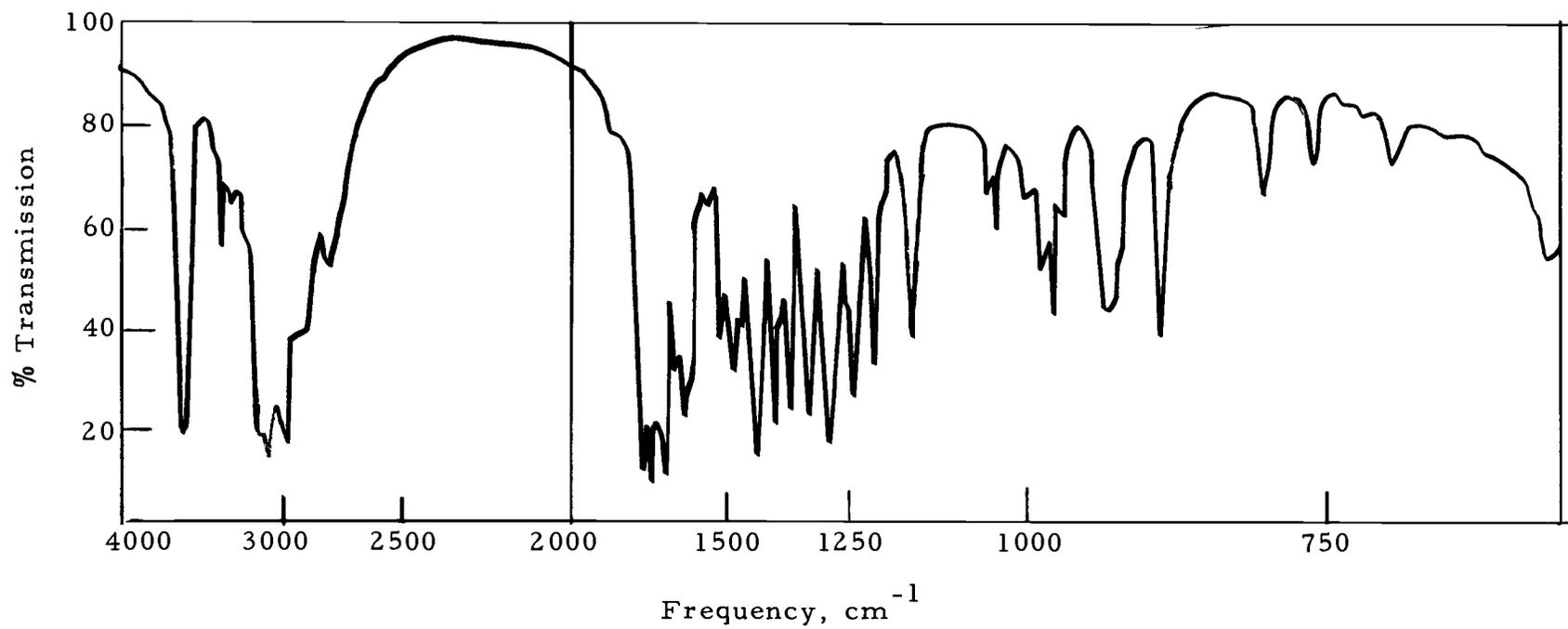
Figure 9. Infrared spectrum of acetylated 2H-K (nujol mull).
