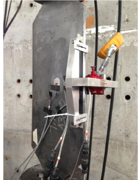
Figure 4-10: Plate test setup in UTM
