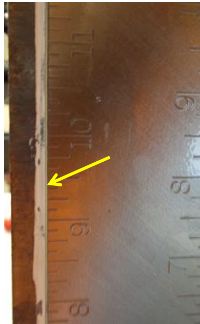
Figure 4-8: No macro-measurable residual deformation of plate after yielding
