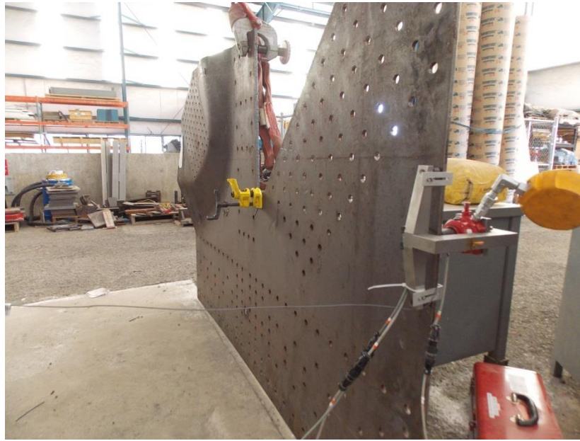
Figure 5-32: Gusset plate test with spare plate in OSU laboratory
