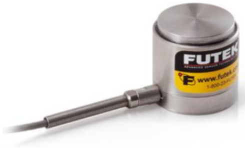
Figure 3-3: Load cell with 10 kip capacity ( http://www.futek.com/product.aspx?t=load&m=lca305 )
