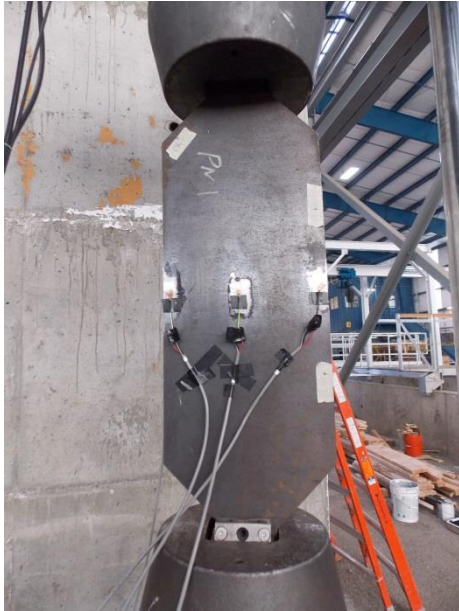
Figure 4-9: Axially loaded plate strain gauge setup
