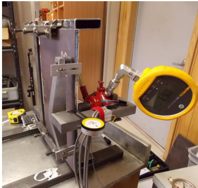
Figure 4-7: Free plate testing setup
