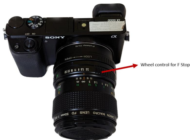
Fig. 7 Moving the wheel control indicated above controls the F Stop setting.
