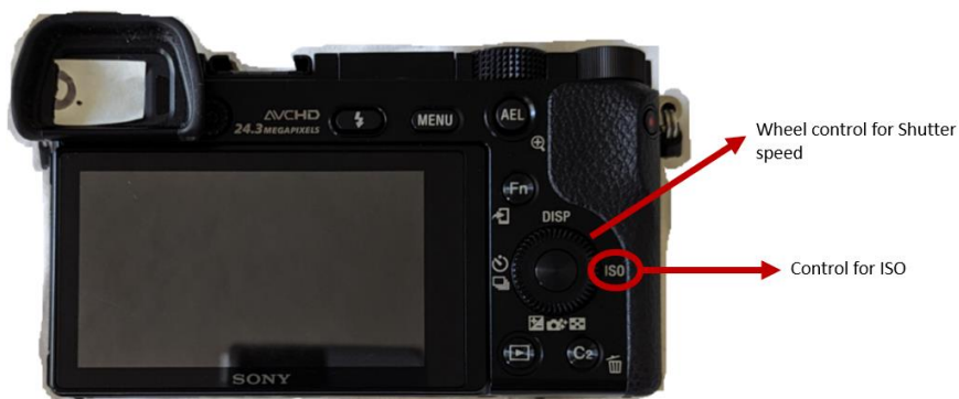
Fig. 8 Scrolling the wheel control changes the shutter speed. Pressing down on the wheel once on the side that says ISO and scrolling the wheel will change the ISO settings.
