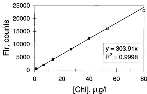
Fig. 5. Fluorescence (Flr) response (violet excitation) as a function of extracted chlorophyll (Chl) concentration. Peak fluorescence values are derived from blank-corrected averaged spectra. Error bars representing the 95% confidence limits ( $\pm 2$  standard errors from the mean) of these measurements lie within the data point character. The linear fit to the data is constrained to include the origin and excludes the data points at the two highest concentrations.
