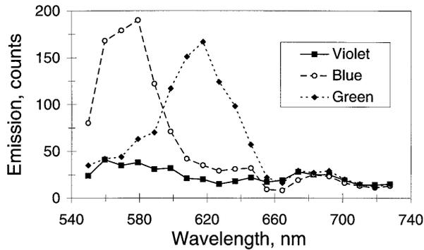
Fig. 4. Water emission spectra: violet, blue, and green excitation. Each spectrum was obtained by averaging 1780 spectra. Error bars representing the 95%-confidence limits ( $\pm 2$  standard errors from the mean) of these measurements lie within the data point character. Water was filtered, distilled, and purified by reverse osmosis. Spectra have not been corrected for the difference in the number of excitation quanta in each excitation channel.
