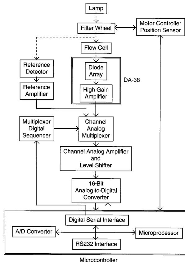
Fig. 3. Electrical block diagram. The dashed lines indicate light path.
