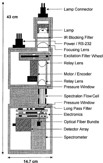
Fig. 1. Fluorometer schematic.
