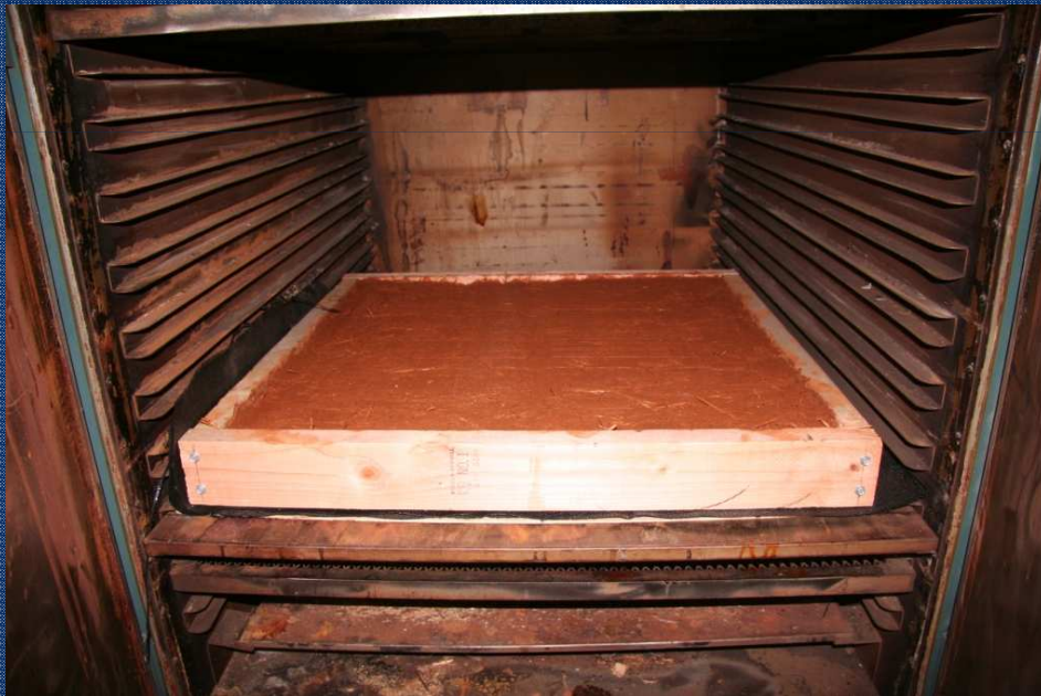
Cob in Oven Prior to Drying
