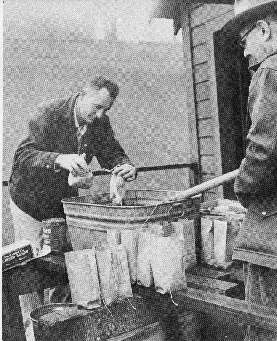
Game Commission personnel try out new balloon method for testing fish loss in turbines. A small plastic capsule containing calcium hydroxide is inserted in a balloon with a small amount of water to dissolve the glue sealing the capsule. The collapsed balloon is tied to the outside of a thin lightweight bag containing live fish. The bag, weighted down with a paper sack of sand, is dropped into the turbines. By the time the bag of fish reaches the raceway below, the capsule has dissolved and the resulting hydrogen gas inflates the balloon, bringing the bag of fish to the surface. Sometimes two balloons are used for each bag to assure better recovery. This method was developed by Ivan Donaldson, biologist with Corps of Engineers.
