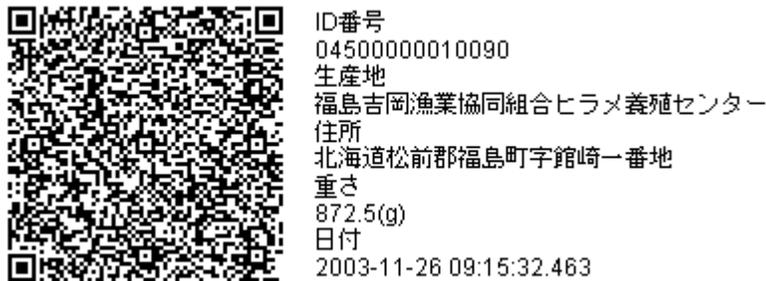
**Figure 2.** An example of a 2D code tag. This tag is designed so that basic information can be read directly by the code and the detail information is retrieved via internet connection by a java application on a mobile phone. Digitally encrypted weight information is included in this tag.
