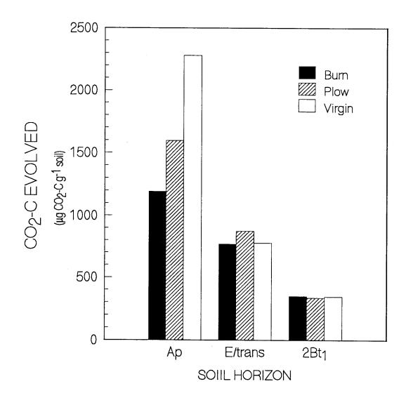
**Figure 3.** Comparison of total CO<sub>2</sub>-C g<sup>-1</sup> soil evolved from microbial respiration during a 32 day incubation period between a virgin soil and soils cropped to annual ryegrass under a burned or plowed straw residue management system.
