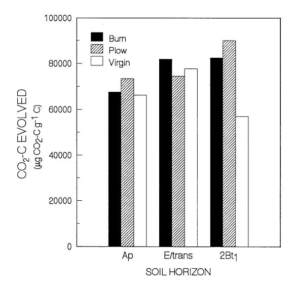
**Figure 5.** Comparison of total CO<sub>2</sub>-C g<sup>-1</sup> carbon evolved from microbial respiration during a 32 day incubation period between a virgin soil and soils cropped to annual ryegrass under a burned or plowed straw residue management system.
