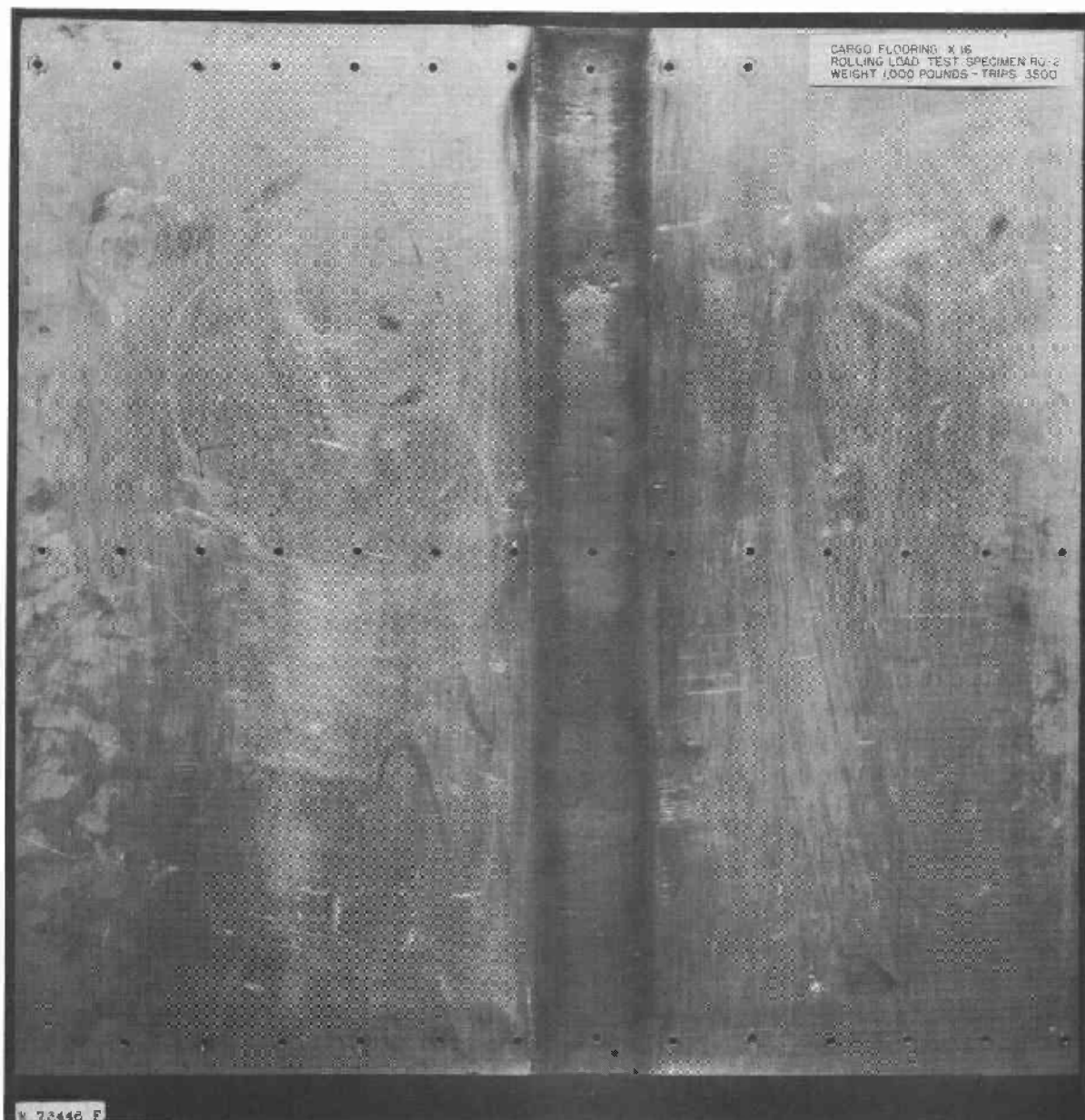
Figure 21.--Upper surface of cargo floor X 16 rolling-load specimen RO-2, showing effect of rolling a 1,000-pound engine-cradle-wheel load over the panel 3,500 trips.
