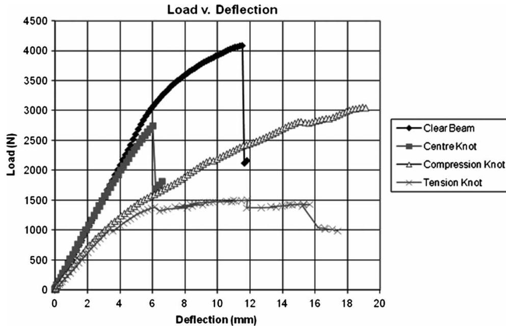
Figure 2. Plot of load versus deflection for each beam.
