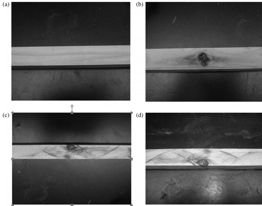
Figure 1. (a) Clear specimen; (b) specimen with a knot at the mid-height of the face; (c) specimen with a knot in compression; (d) specimen with a knot in tension.
