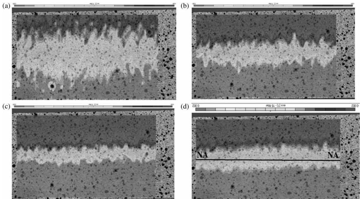
Figure 5. Longitudinal strain contour plots for a clear beam under (a) 0.997 kN load; (b) 2.01 kN load; (c) 3.03 kN load; and (d) failure load: 4.08 kN.
