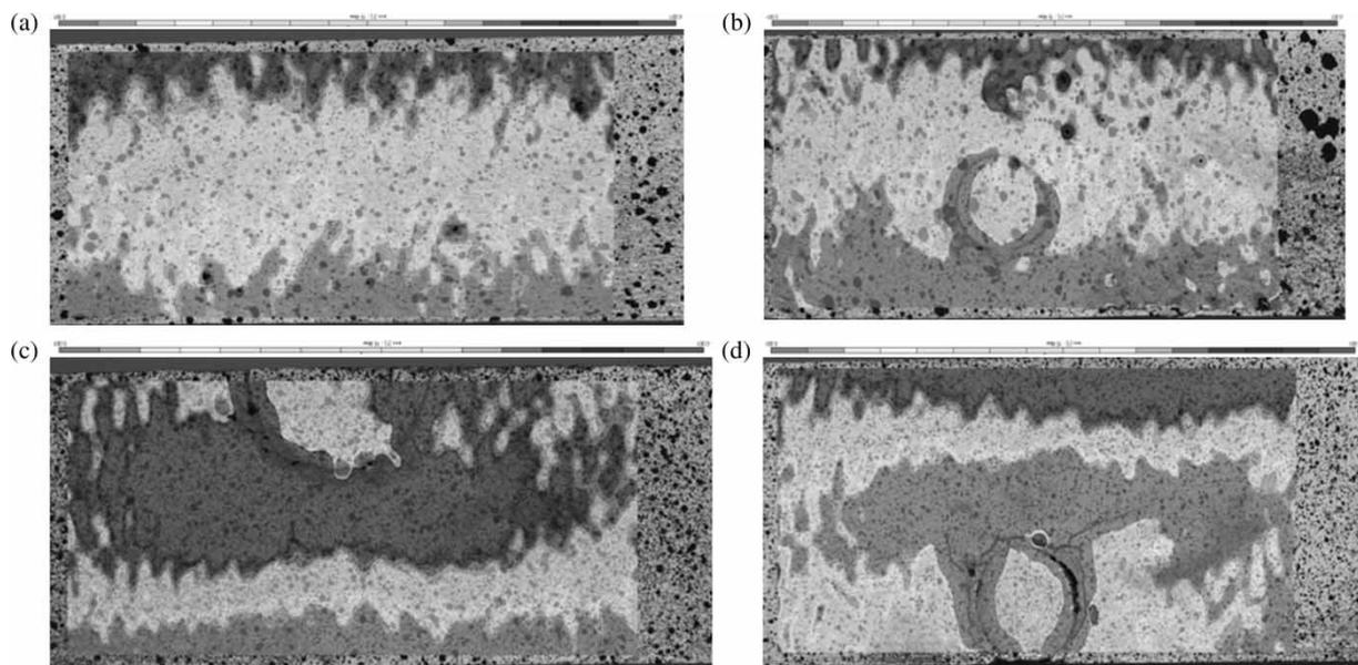
Figure 3. Longitudinal strain contour plots at elastic state (load  $\approx$  730 N) for: (a) clear beam; (b) knot located at centre; (c) knot located in compression zone; and (d) knot located in tension zone.
