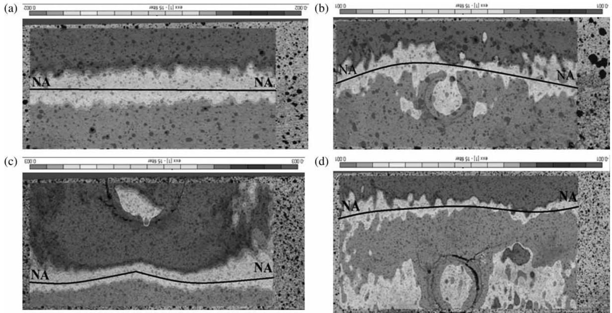
Figure 4. Longitudinal strain contour plots just before failure for: (a) clear beam; (b) knot located at centre; (c) knot located in compression zone; and (d) knot located in tension zone.
