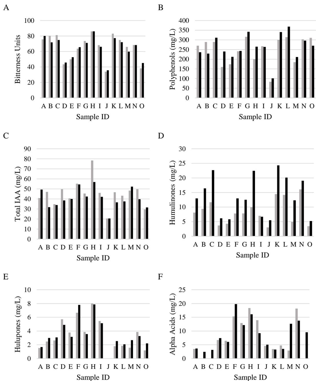
Figure 13. The impact of dry-hopping for pre-dry-hop (gray) and post-dry-hop (black) on (A) bitterness units, (B) polyphenols (mg/L), (C) total IAA (mg/L), (D) humulinones (mg/L), (E) hulupones (mg/L), and (F) alpha acids (mg/L).
