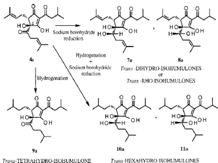
Figure 5. Production of reduced isohumulones. (28)
