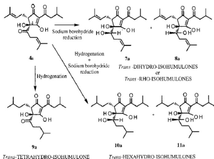
Figure 5. Production of reduced isohumulones. (28)
