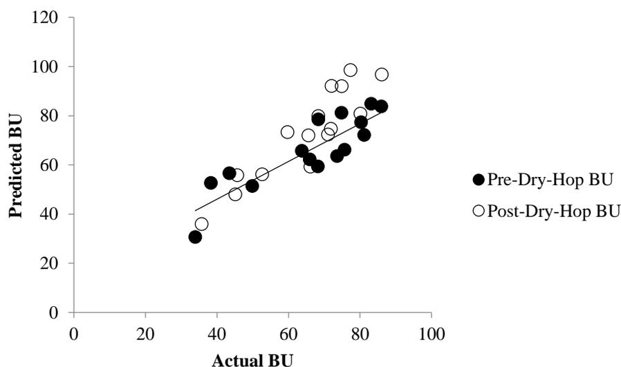
Figure 12. Predicted BU vs. actual BU values using the pre-dry-hop multiple linear regression model. The trendline indicates the slope of the pre-dry-hop BU values.
