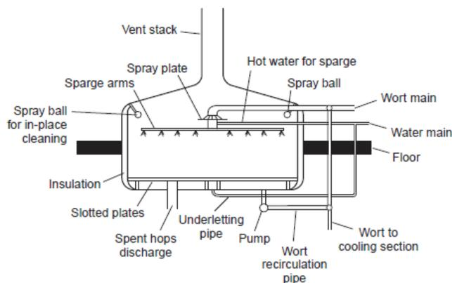
Figure 2. Diagram of a hop back. (4)
