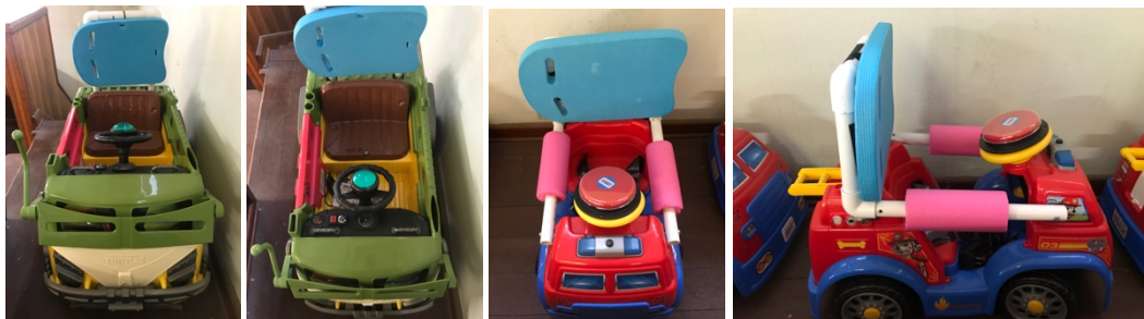
Figure 1. Images of Modified Ride-On Cars with easy-to-use push button and safety protections.
