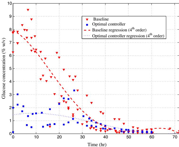
**Fig. 9** Comparison of glucose concentrations: optimal control vs baseline
