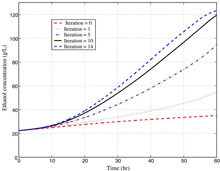
**Fig. 8** Predicted ethanol concentrations (g/L) for different optimal profiles
