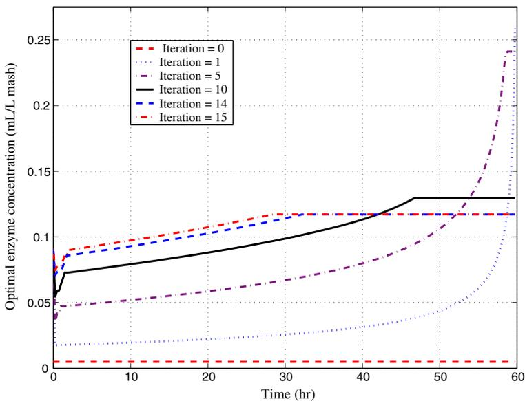
Fig. 6 Predicted glucoamylase enzyme dose profiles as a function of iteration number
