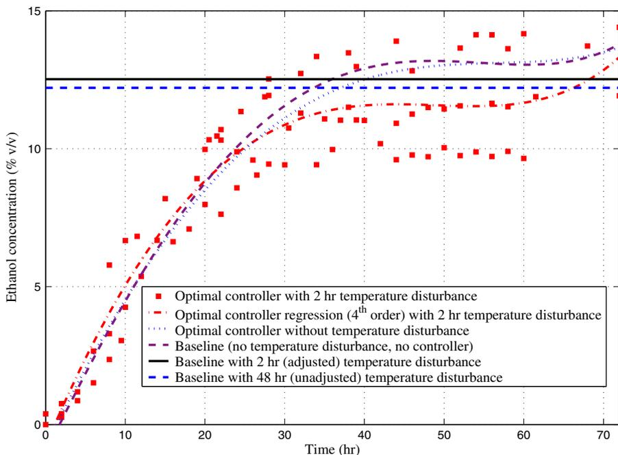
**Fig. 12** Comparison of ethanol concentrations: temperature perturbation vs baseline
