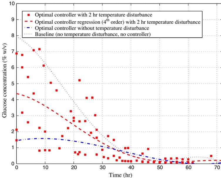
**Fig. 11** Comparison of glucose concentrations: temperature perturbation vs baseline
