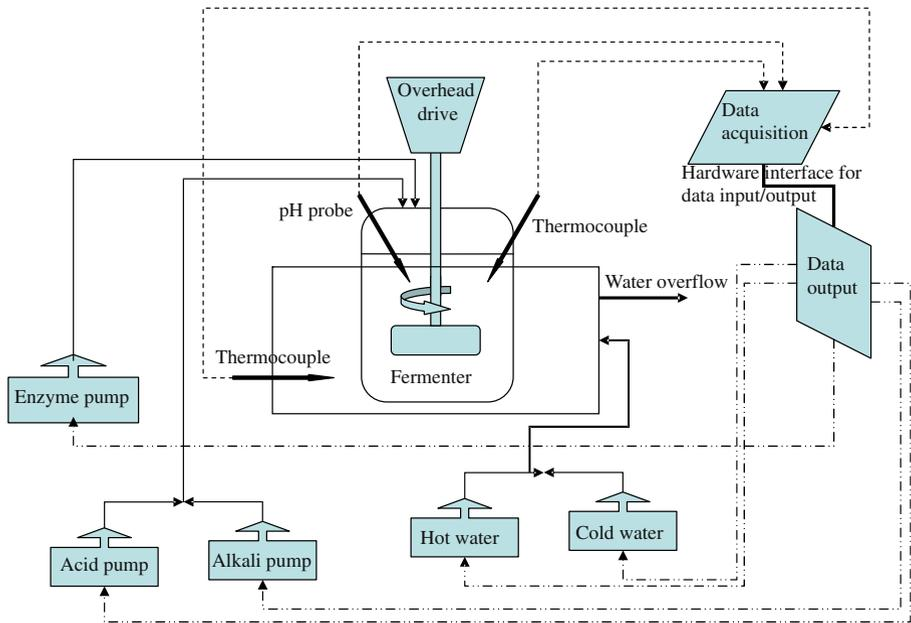
**Fig. 3** Schematic of the fermentation system to evaluate optimal controller
