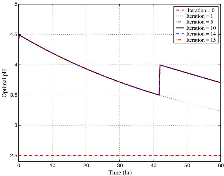
Fig. 5 Predicted pH profiles as a function of iteration number
