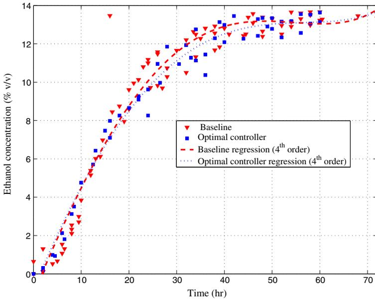
**Fig. 10** Comparison of ethanol concentrations: optimal control vs baseline
