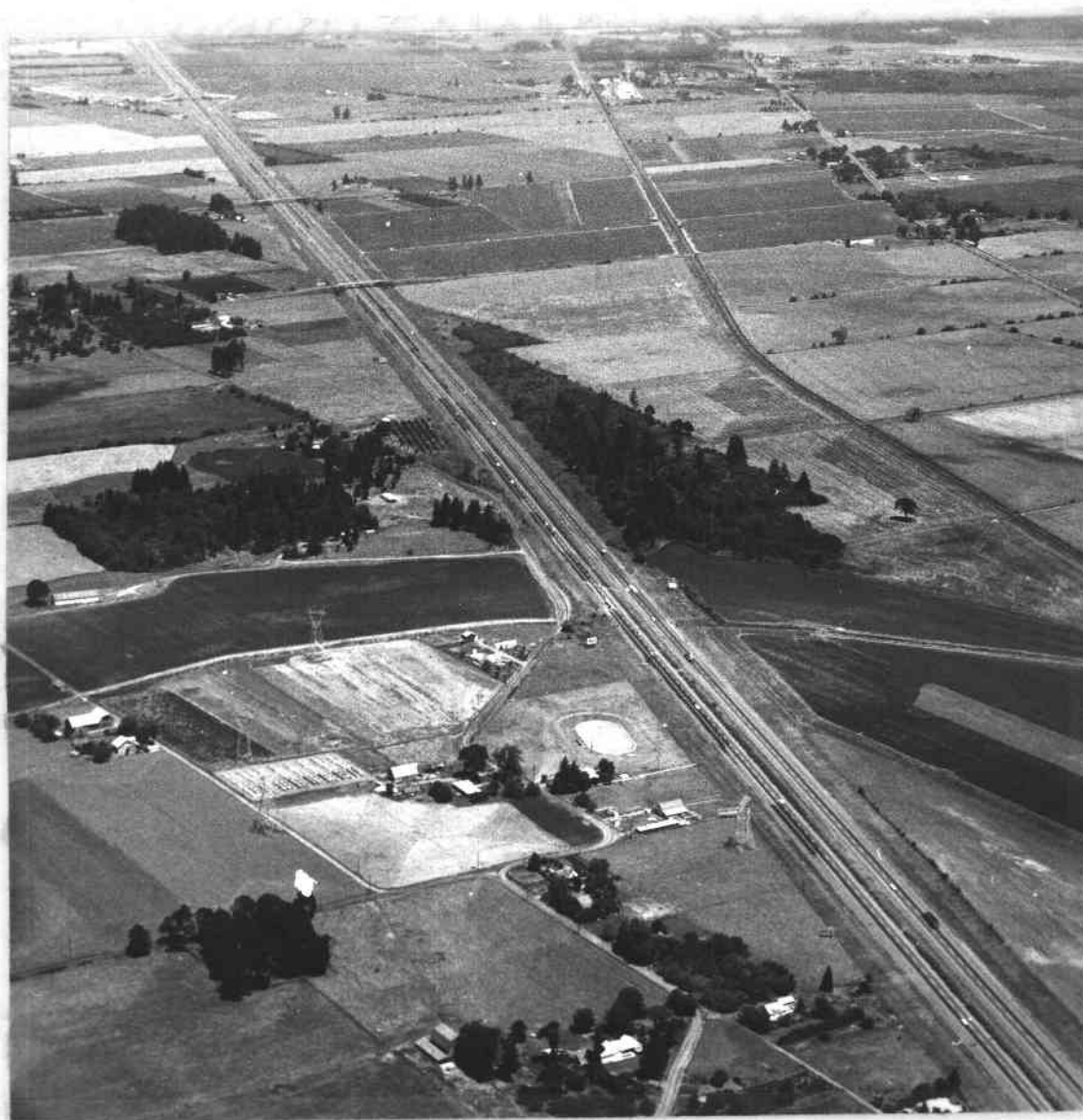
Figure 5. The Hayesville to Nyberg segment of Interstate 5, illustrating the smooth, level topography of the southern portion of the study area. Note the reflection of topography in the nature of freeway construction, with this portion of Interstate 5 utilizing a median strip to separate the north and south bound lanes of traffic.
