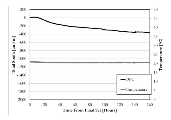
Figure 6-4: Autogenous deformation and temperature of OPC mortar sample
