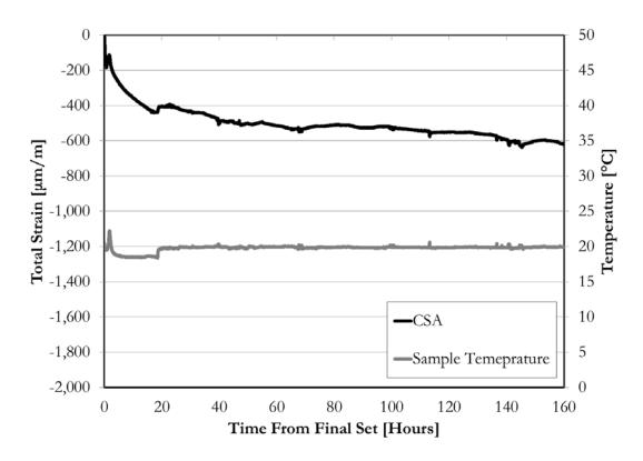
Figure 6-3: Autogenous deformation and temperature of CSA mortar sample
