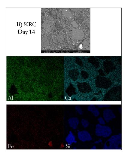
Figure 5-9: SEM image and elemental map of Al, Ca, Fe, and Si from EDX for KRC mixture day A) 1 and B) 14
