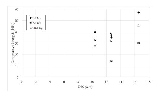
Figure B-3: 1, 3, and 28-day compressive strengths against coarse aggregate D50 values
