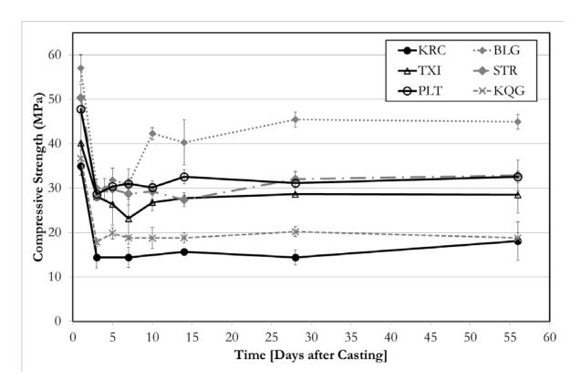
Figure 5-3: Compressive strength of concrete mixtures containing siliceous aggregates
