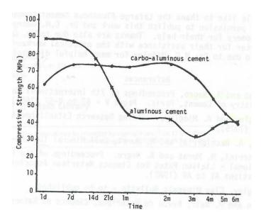
Figure 1-6: Compressive strengths of 100% CAC ("aluminous cement) and 70%CAC/30% FGLS (carbo-aluminous cement) pastes cured for 24 hours at 20°C followed by long-term curing at 38°C [80]
