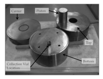
Figure 2-5: Disassembled pore solution extraction dye system
