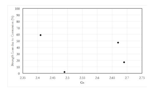
Figure B-8: Percent strength reduction due to conversion against fine aggregate G<sub>s</sub> values
