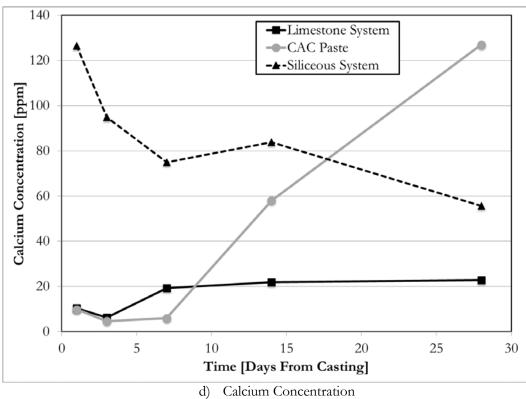
**Figure 4-1:** Elemental concentration (1a-1d) of CAC concrete and paste systems over time when subjected to accelerated conversion curing regime
