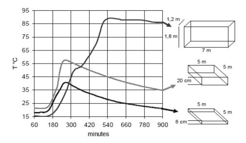
Figure 1-4: Internal temperature in different sized CAC concrete elements[11]
