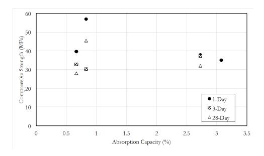
Figure B-13: 1, 3, and 28-day compressive strengths against coarse aggregate absorption capacity values
