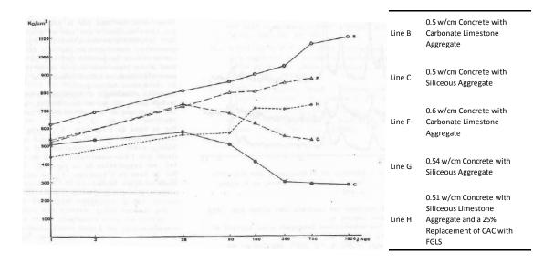
Figure 1-10: Concrete compressive strength results from Cussino and Negro (Translated from original French) [91]
