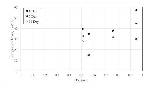
Figure B-1: 1, 3, and 28-day compressive strengths against fine aggregate D50 values
