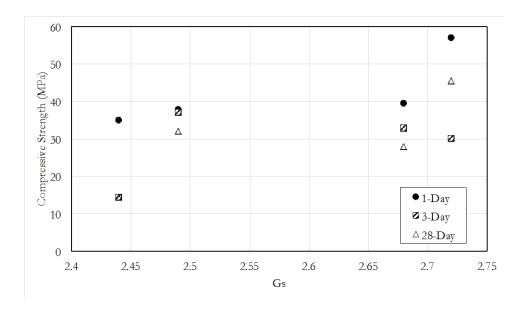
Figure B-9: 1, 3, and 28-day compressive strengths against coarse aggregate G<sub>s</sub> values
