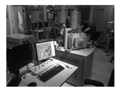
Figure 2-11: FEI Quanta 600F environmental SEM
