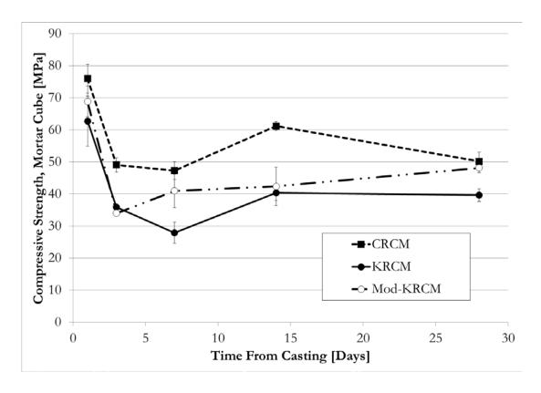
Figure 5-6: Compressive strengths in micro-concrete mixtures
