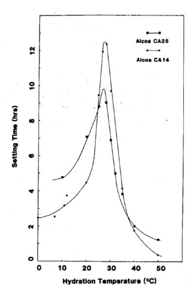
Figure 1-7: Effect of temperature on setting time of CAC paste [55]
