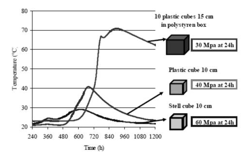
Figure 1-5: Impact of mold type on self-heating on CAC concrete [11]
