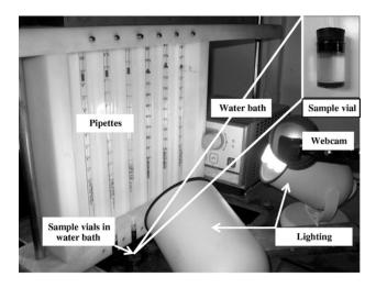
Figure 2-2: Automated chemical shrinkage monitoring apparatus [19]
