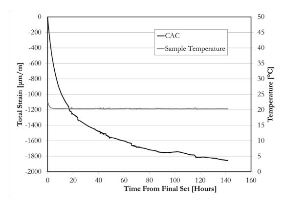
Figure 6-2: Autogenous deformation and temperature of CAC mortar sample
