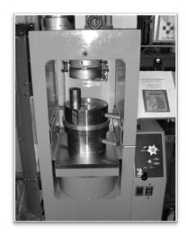
Figure 2-6: Assembled pore solution extraction dye system placed in compression machine
