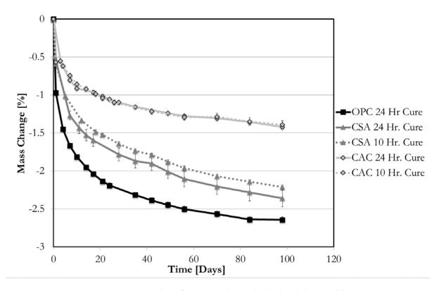
Figure 6-7: Mass loss of concrete prisms submitted to drying conditions
