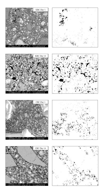
Figure 5-2: Example original SEM image (left) and segmented image (right) from KRC and CRC mixtures at 1 and 14 days
