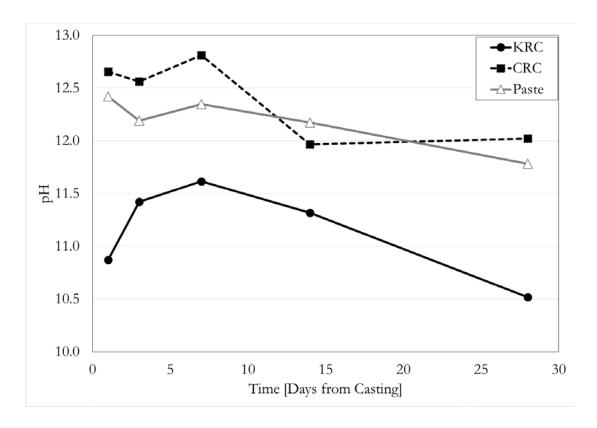
Figure 5-8: pH of pore solution of CRC, KRC, and Paste mixtures
