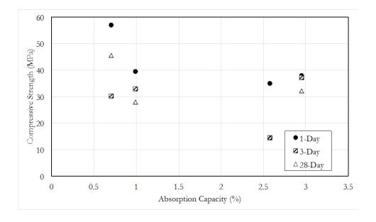
Figure B-11: 1, 3, and 28-day compressive strengths against fine aggregate absorption capacity values
