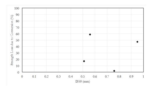
Figure B-2: Percent strength reduction due to conversion against coarse aggregate D50 values
