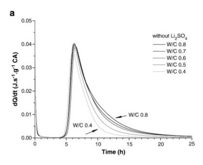
Figure 1-2: Heat flow curve of CAC Hydrated at 20°C [76]
