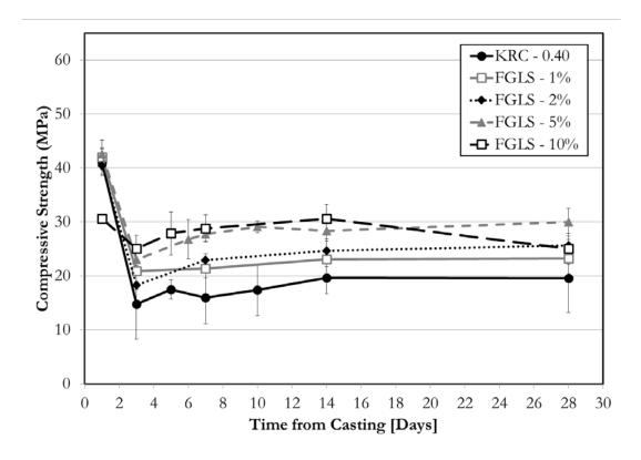
Figure 3-7: Compressive strength of CAC systems incorporating FGLS
