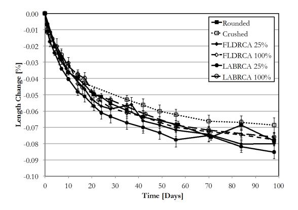
Figure A-3: Length change due to drying of concrete prisms
