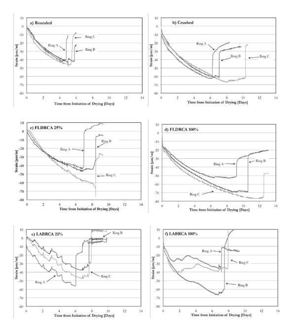
Figure A-5: Restrained shrinkage ring results for all mixtures
