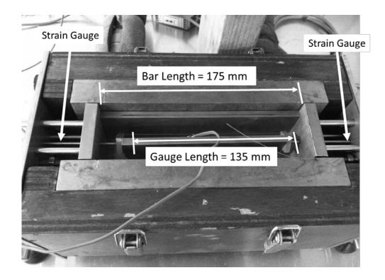
Figure 2-3: Interior of the free deformation frame
