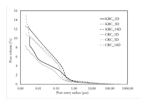
Figure 5-12: Porosity development as determined by MIP
