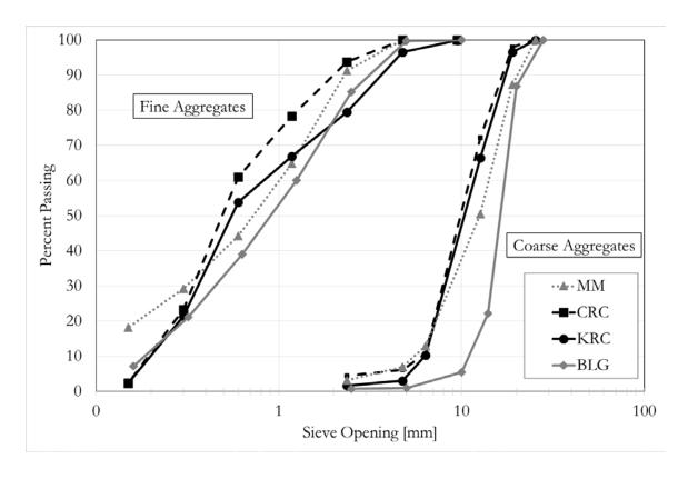
Figure 5-1: Sieve analysis results for selected coarse and fine aggregates
