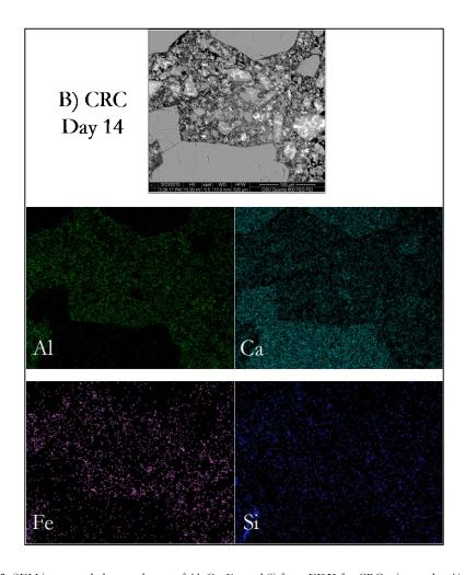
Figure 5-10: SEM image and elemental map of Al, Ca, Fe, and Si from EDX for CRC mixture day A) 1 and B) 14
