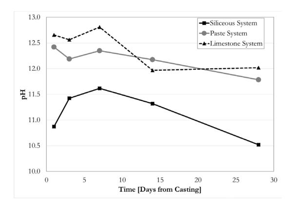
Figure 4-2: pH evolution of CAC concrete and paste systems over time when subjected to accelerated conversion curing regime
