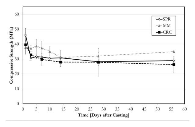
Figure 5-4: Compressive strength of concrete mixtures containing limestone aggregates
