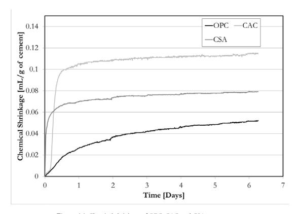
Figure 6-1: Chemical shrinkage of OPC, CAC, and CSA cement pastes
