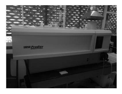
Figure 2-7: ICP-OES apparatus used in this work
