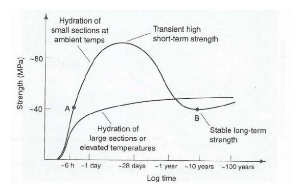
Figure 1-8: Effect of conversion on strength in CAC systems[4]
