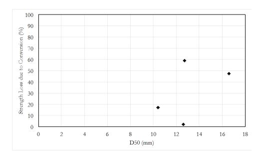
Figure B-4: Percent strength reduction due to conversion against coarse aggregate D50 values
