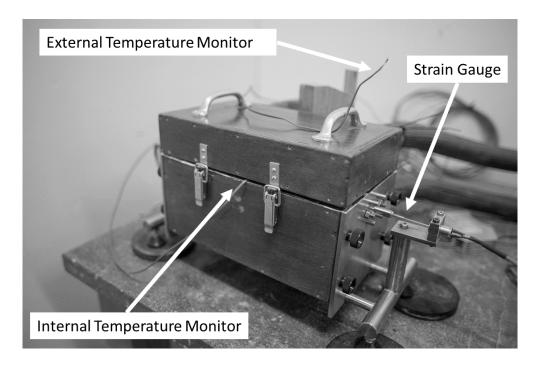
Figure 2-4: Exterior of closed and sealed free deformation frame
