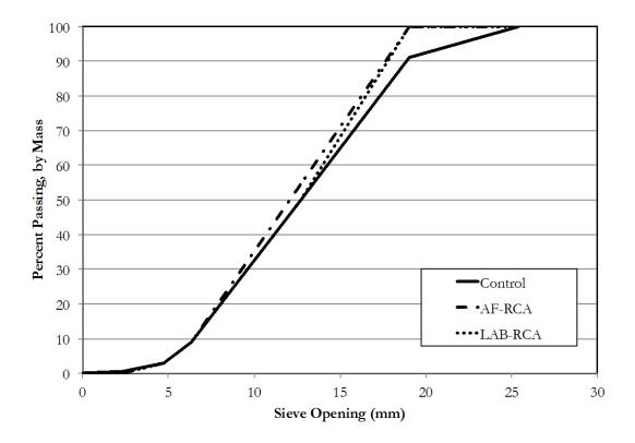
Figure A-2: Grading of coarse RCA and control aggregates
