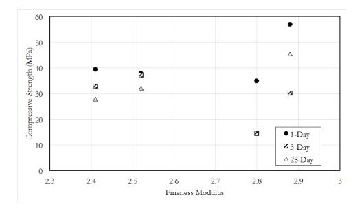
Figure B-5: 1, 3, and 28-day compressive strengths against fine aggregate FM values
