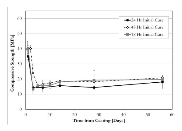
Figure 3-4: Compressive strengths of systems examining length of Phase 1 curing
