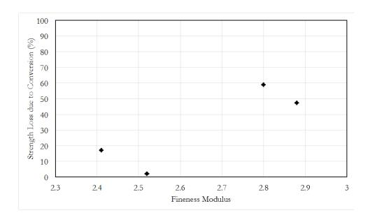
Figure B-6: Percent strength reduction due to conversion against fine aggregate FM values
