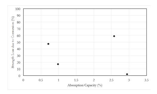
Figure B-12: Percent strength reduction due to conversion against fine aggregate absorption capacity values
