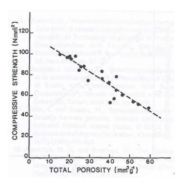
Figure 1-9: Correlation between porosity and compressive strength in CAC mortars as a function of w/cm [90]
