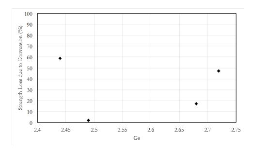
Figure B-10: Percent strength reduction due to conversion against coarse aggregate G<sub>s</sub> values
