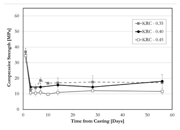
Figure 3-3: Effect of w/cm on time to minimum strength
