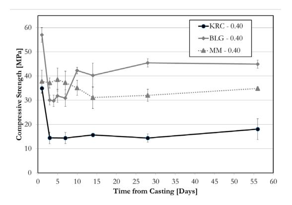
Figure 3-1: Aggregate impact on strength and conversion in CAC concrete
