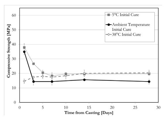
Figure 3-5: Compressive strengths of systems examining temperature of Phase 1 curing
