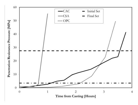
Figure 6-5: Setting time of CAC, CSA, and OPC mortar samples at 20°C
