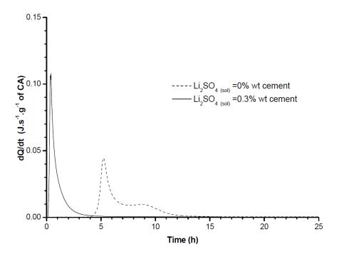
Figure 1-3: Heat flow curve of CAC Hydrated at 38<sup>o</sup>C [45]
