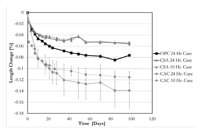
Figure 6-6: Length change of concrete prisms submitted to drying conditions
