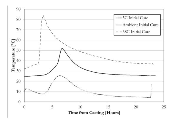
Figure 3-6: Temperature profile for KRC - 0.40 cured at different temperatures during Phase 1
