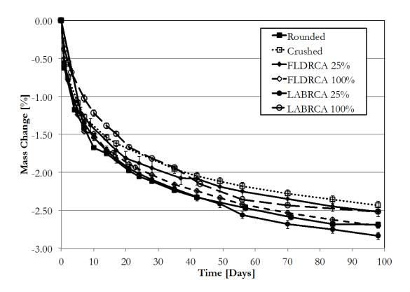
Figure A-4: Mass change due to drying of concrete prisms
