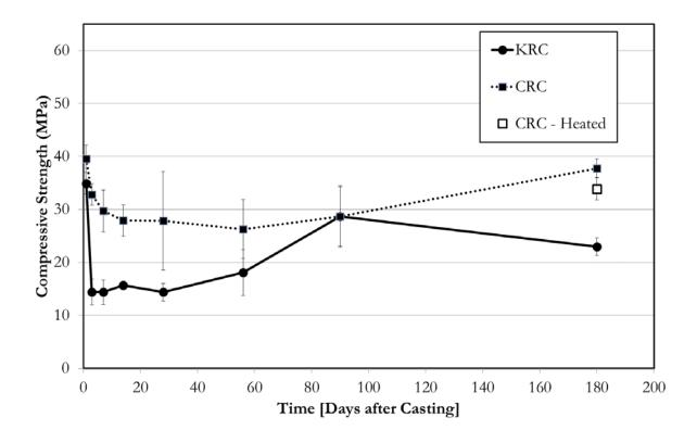
Figure 5-5: Long-term compressive strength of KRC and CRC mixtures
