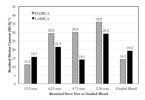
Figure A-1: Residual mortar content (RMC) values of FLDRCA and LABRCA
