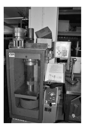
Figure 2-1: Forney FHS-700 used to measure mechanical properties
