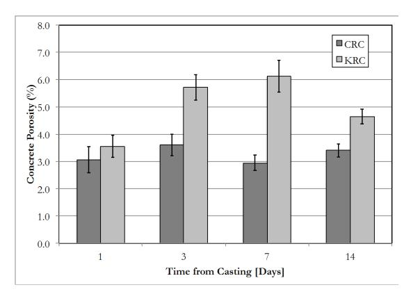
Figure 5-11: Concrete porosity of CRC and KRC mixtures as measured by image analysis
