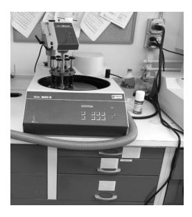
Figure 2-10: LaboPol-35 polishing system with LaboForce-1 counter rotation sample holder
