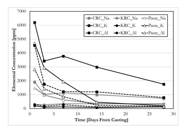
Figure 5-7: Elemental concentration of Na, K, and Al in pore solution of CRC, KRC, and Paste mixtures
