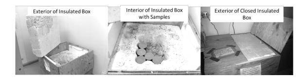
Figure 1-11: Heavily insulated box for curing CAC concrete samples
