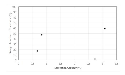
Figure B-14 Percent strength reduction due to conversion against coarse aggregate absorption capacity values
