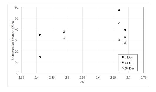
Figure B-7: 1, 3, and 28-day compressive strengths against fine aggregate  $G_{\text{\tiny S}}$  values
