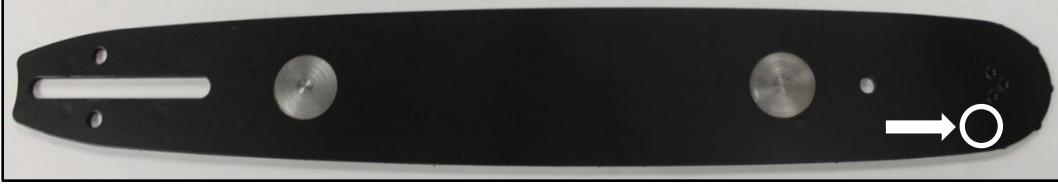
Figure 8: Guide bar prepared for infrared photography. The superimposed arrow and circle show the thermal region of interest selected for comparison in this study.
