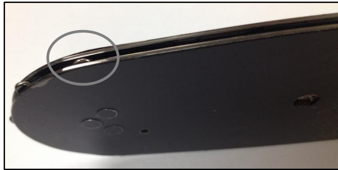
Figure 10: Typical heavy wear at the nose tangency.
