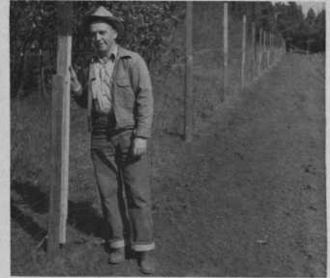
In this salt-treated fence more than half the posts were still firm after 15 \frac{1}{2} years. The peeled tops had not rotted noticeably. Butts were not peeled. Posts were round, Douglas-fir, many small like ones shown. The 2x4 uprights were nailed to the posts to provide a deer fence. Vern McDaniel (shown here), Superintendent, Oregon Forest Nursery, treated the posts.
