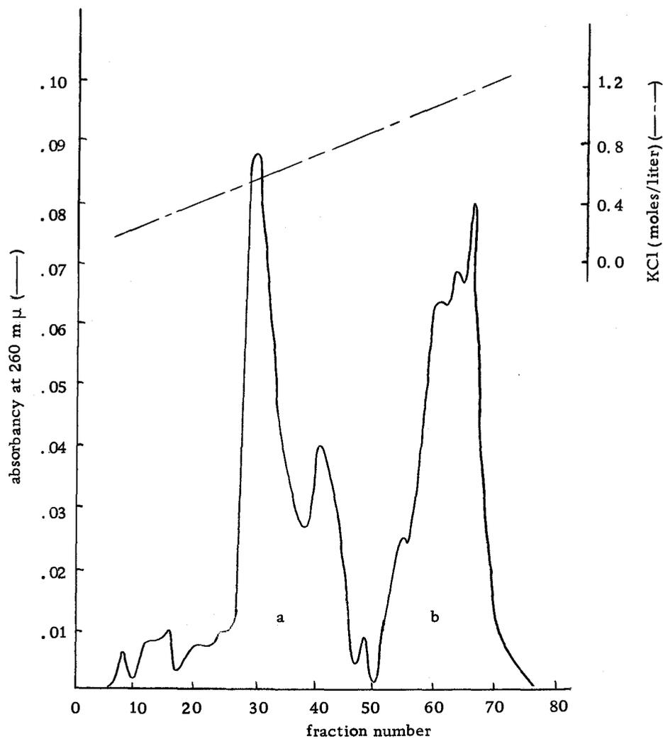
Figure 11. MAK column analysis of fragmented virus RNA preparation. Virus RNA, fragmented during phenol extraction, was applied to the column and eluted with a 0.2-1.2 M KCl gradient in 0.05 M phosphate buffer pH 6.7.
