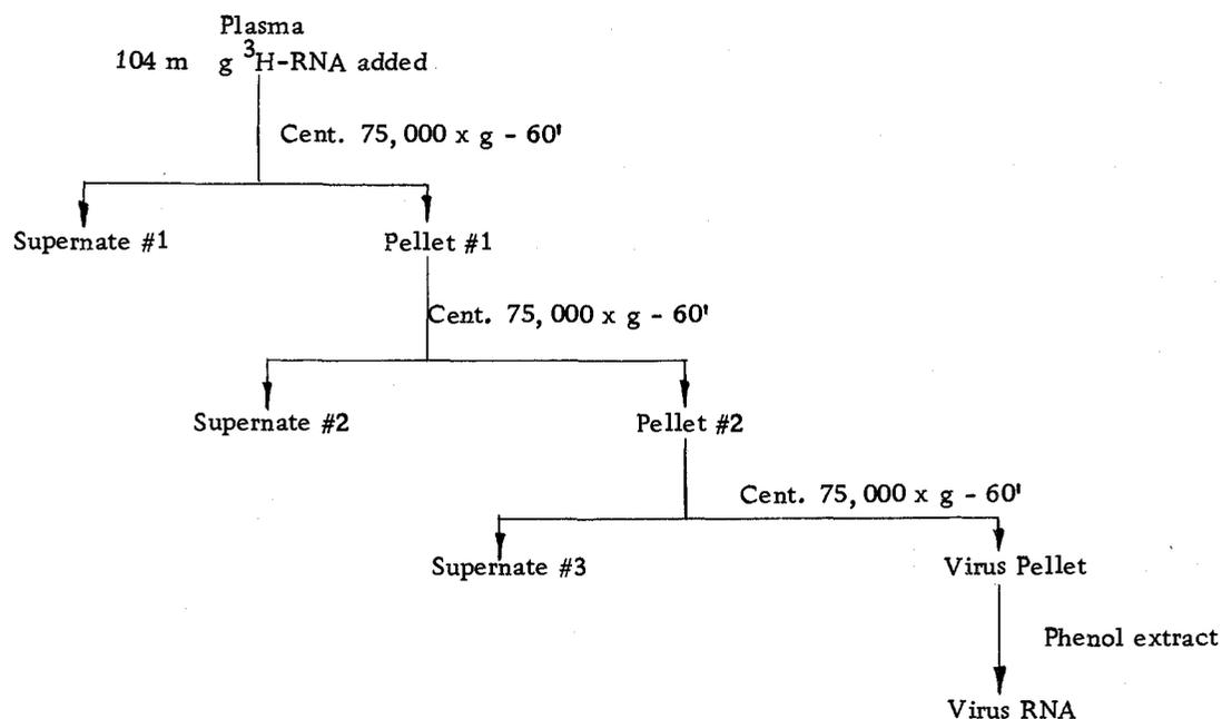
Figure 10. Schematic diagram of virus RNA isolation to determine extraviral RNA contamination.
