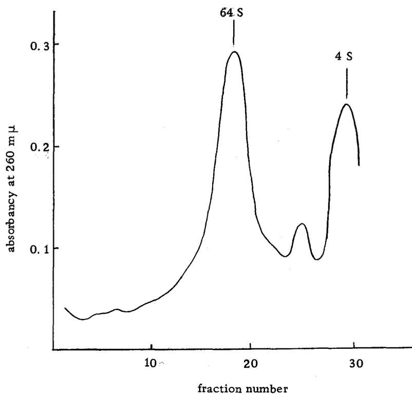
Figure 4. Fractionation of myeloblastosis virus RNA by sucrose density gradient centrifugation. Myeloblastosis virus RNA was layered on top of a 5-20% sucrose gradient (sucrose solution was in 0.01 M tris buffer, pH 7.8, 0.1 M NaCl, 0.001 M EDTA) and centrifuged in a SW 25.1 rotör, Spinco Model L, for four hours at 25,000 rev./min.
