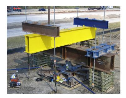
Figure 4.10 Load test setup for a large footing after Stuedlein (2008), using helical anchors as reaction.
