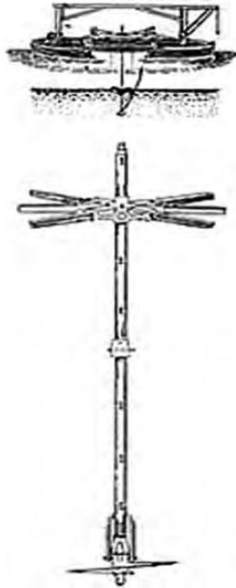
**Figure 2.3 Mitchel screw pile (Perko, 2009).**
