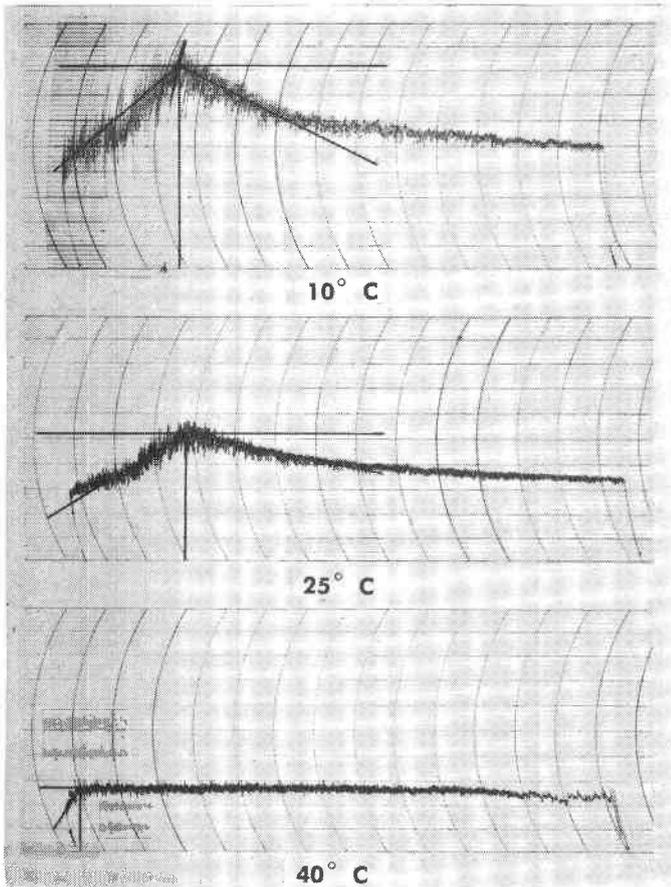
Figure 1. Mixograms made at different temperatures.
