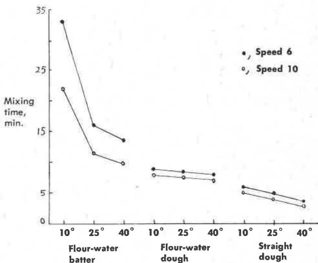
Figure 4. Total mixing time required for gluten development. Times given include preliminary mixing at different speeds and temperatures and final mixing to develop bread dough.
