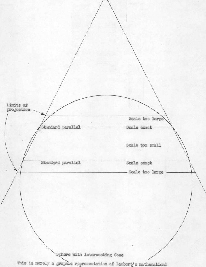
This is merely a graphic representation of Lambert's mathematical projection based on Clarke's spheroid of 1866.
