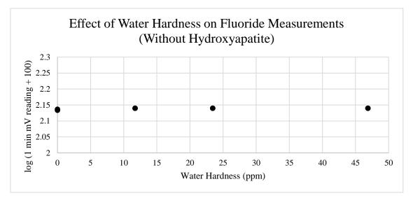
Figure 6: When fluoride ions are exposed to hard water without nano-hydroxyapatite, there is no significant difference in the readings of fluoride.
