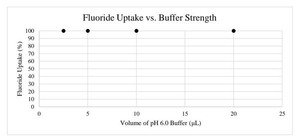
*Figure 8: The buffer strength does not affect nano-hydroxyapatite's uptake of fluoride ions during a 90-minute exposure.*
