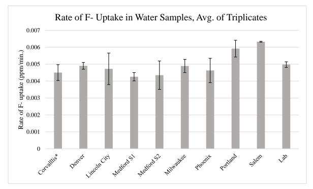
Figure 9: The rate of fluoride ion uptake does not significantly vary between water samples between different cities. Average values for each city are plotted, and the error bars represent the standard deviation for each set of samples. \*Note: Due to an unknown experimental error, Trial 1 of Corvallis' sample was thrown out.
