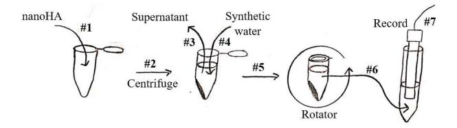
Figure 1: A generalized model for fluoride exposure testing.
