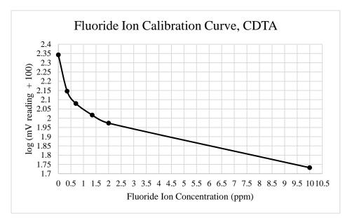
Figure 2: A representative calibration curve, used to determine the concentration of fluoride ions in a solution. Calibration curves were frequently remeasured and never appreciably differed from the sample shown here.
