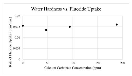
Figure 5: During a 20-minute exposure period, the water hardness does not significantly affect hydroxyapatite's uptake of fluoride ions. Note that, in addition to calcium carbonate, the synthetic hard water also contained magnesium chloride and sodium bicarbonate, as described in the text.
