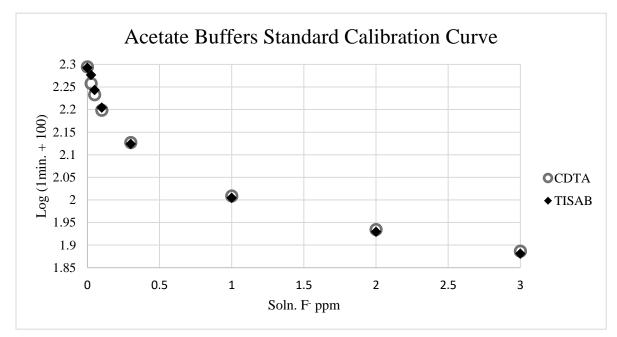
*Figure 3: There is no significant difference in fluoride readings between using TISAB buffer and CDTA buffer.*
