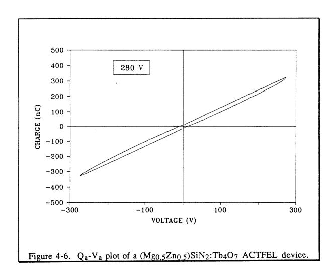
This formulation is now employed to assess the  $(Mg_{0.5}Zn_{0.5})SiN_2:Tb_4O_7$  ACTFEL device of Fig. 4-4. Using the new notation,  $C_i=C_i$ "=6.23 nF and  $C_p=C_p$ "=1.82 nF from  $\varepsilon_i$ =18,  $\varepsilon_p$ =11,  $d_i$ =2200 angstrom,  $d_p$ =4600 angstrom, and A=0.086 cm<sup>2</sup>. Inserting  $C_i$ =6.23 nF and  $C_i$ '=1.5 nF in Eqn. 4-3 yields  $C_p$ =1.97 nF. Comparing  $C_p$  to  $C_p$ , it is seen that  $C_p$ z is quite close to  $C_p$ ; therefore it can be
