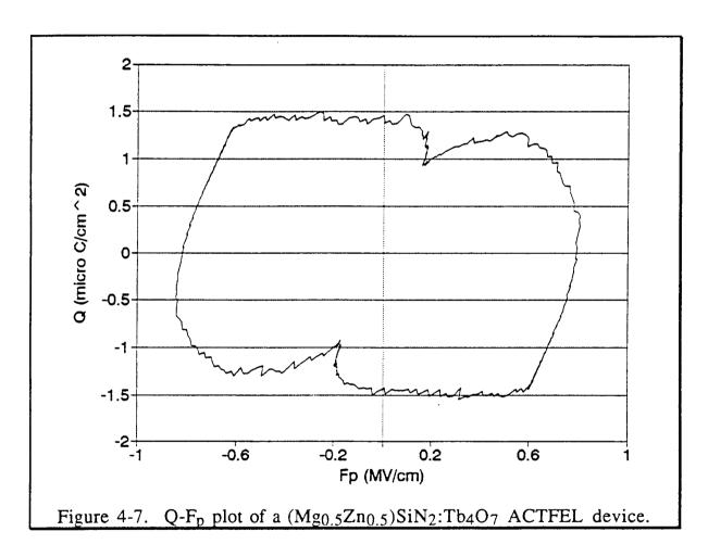
concluded that the  $(Mg_{0.5}Zn_{0.5})SiN_2:Tb_4O_7$  phosphor is only weakly broken down.
