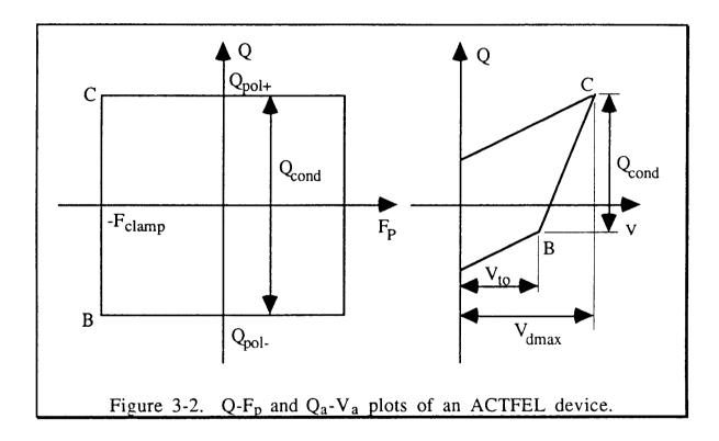
The electrostatic boundary condition at point C in Fig. 3-2 requires that
