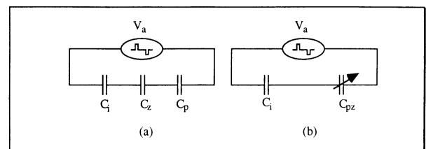
Figure 4-5a. An equivalent circuit of an ACTFEL device with a ZnS injector layer, prior to breakdown.
