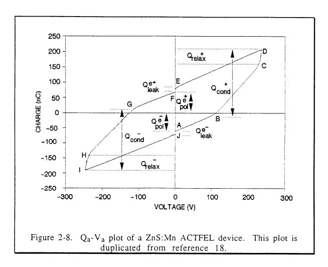
From the  $Q_a$ - $V_a$  and Q- $F_p$  plots, it is seen that when the pulse voltage is zero, i.e. point A, the charge is not zero. This charge is due to electrons which remain trapped at interface states, this is the polarization charge left behind after the previously applied negative
