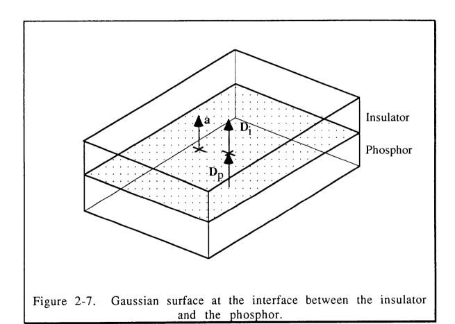
Figure 2-7 shows a Gaussian surface, which is a surface between the insulator and the phosphor of an ACTFEL device. After evaluating the surface integral, Eqn. 2-1, the internal charge is given by,
