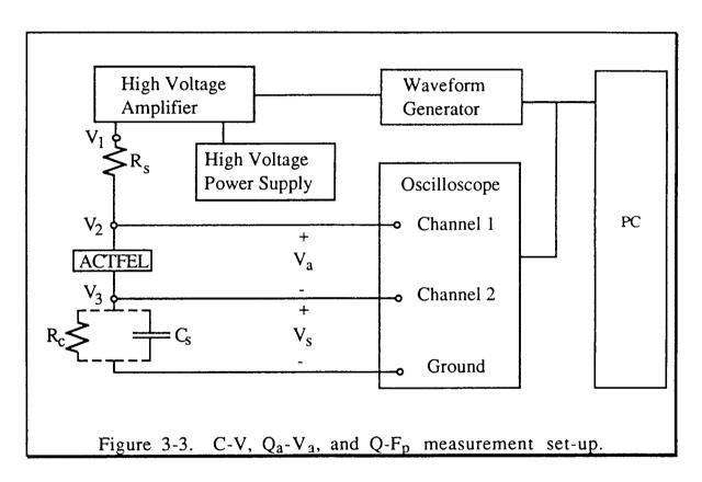
series with the ACTFEL device to prevent device burn out. This series resistor also protects the waveform driver when an ACTFEL device burns out.
