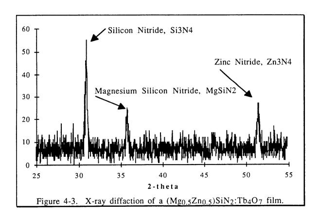
X-ray diffraction results for films after post-deposition annealing at 500 C, 600 C, 650 C, and 700 C are similar to that of the as-deposited film. Thus, there is no sign of crystal structure enhancement due to post-deposition annealing.
