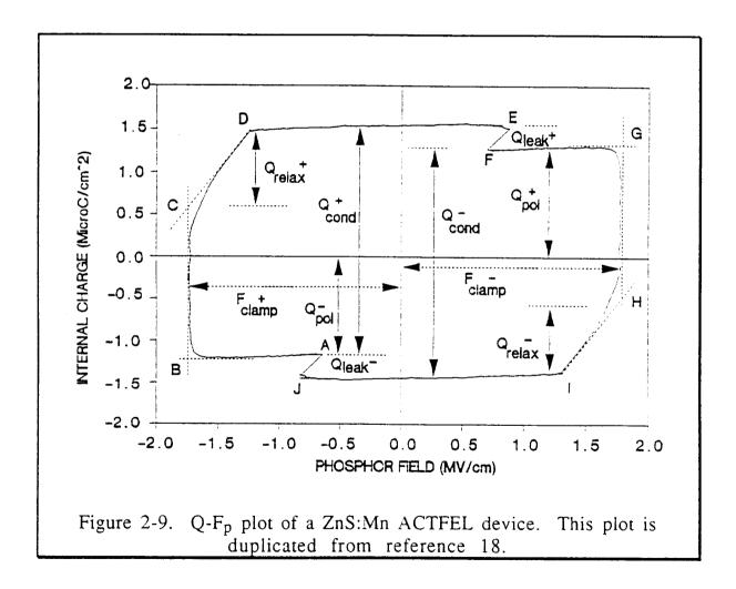
As the applied voltage reaches the turn-on voltage, i.e. point B, electrons at interface states begin tunnel injection into the phosphor conduction band, leaving behind a positively charged interface. As
