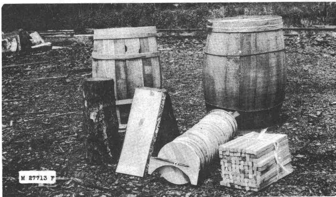
Fig. 4.--Potato barrel, fish barrel, hamper bottoms, and cleats made from small pine.
