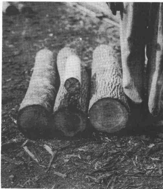
Fig.10.--Small black gum veneered to a 3-3/4-inch core at one mill.
