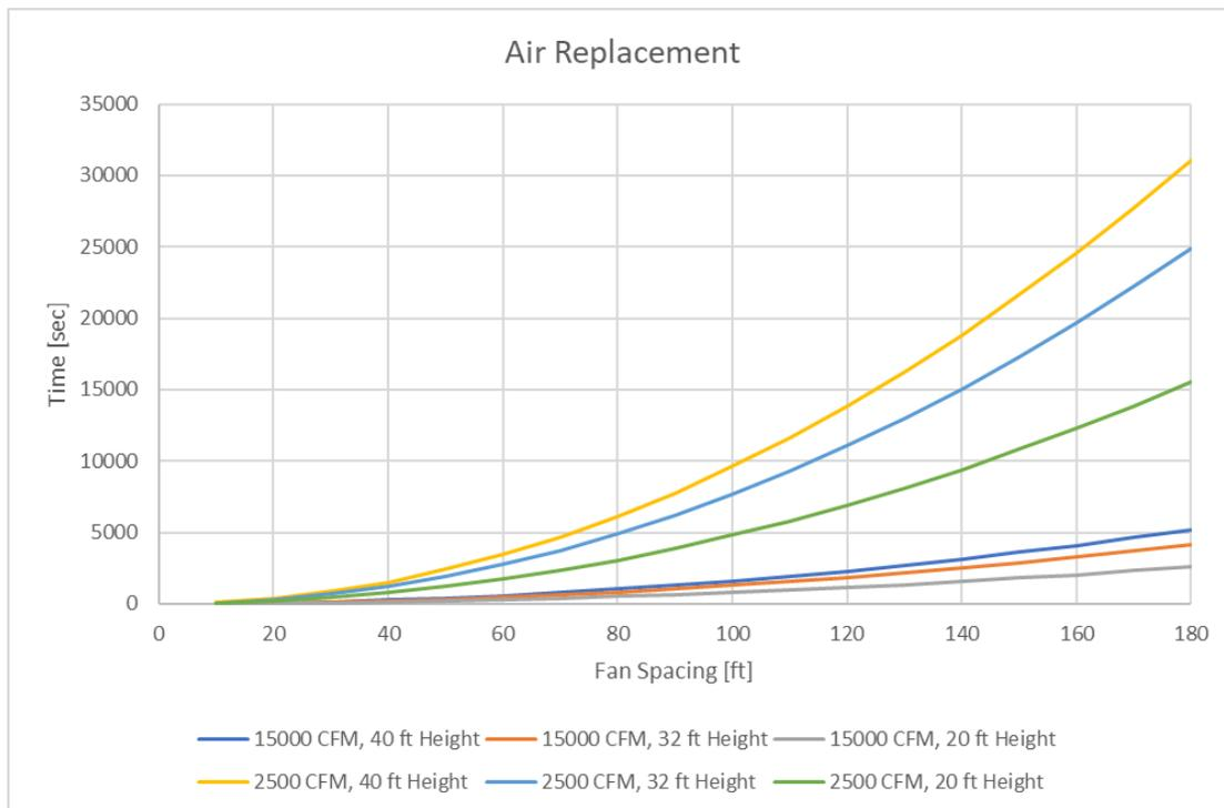
Figure 7.3: Time for air replacement at variable fan spacing
