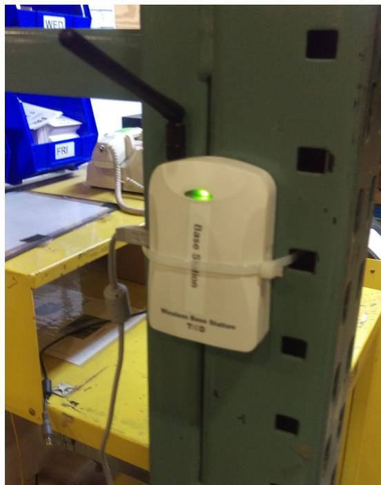
Figure 3.8: Base unit RTR 500 repeater
