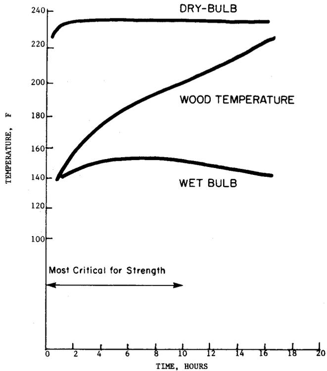
Figure 1 -- Temperature history for SYP 2 x 4's dried at high temperature.
