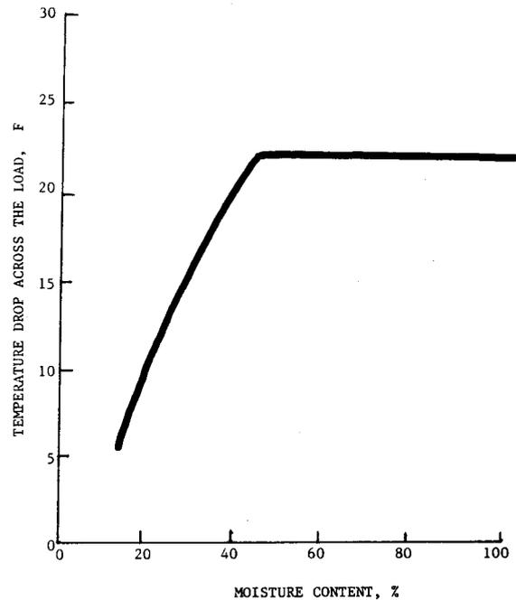
Figure 2 -- TDAL vs. MC in a Commercial Kiln Drying SYP 2 x 4's.
