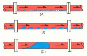
It has been proven that the theoretical figure of 54 psi for each foot per second of velocity that is stopped by a valve is essentially correct, and with the closure of a valve, a pressure of 540 psi above system pressure is possible with a flow velocity of 10 feet per second.
