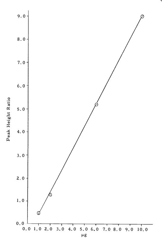
Figure 2. Standard Curve for Ephedrine Hydrochloride
