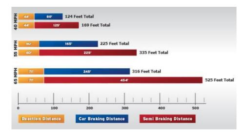
Figure 1.2: Total Stopping Distances at Various Speeds (Source: Utah Department of **Transportation**, 2018)
