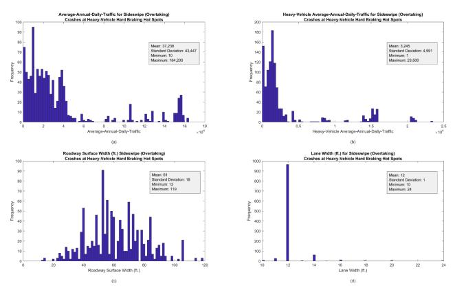
Figure 3.22: (a) AADT, (b) T-AADT, (c) Roadway Surface Width, and (d) Lane Width for Sideswipe (Overtaking) Crashes
