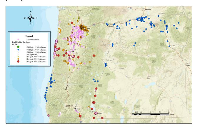
Figure 3.5: Rear-End Crashes at Heavy-Vehicle Hard Braking Hot Spots
