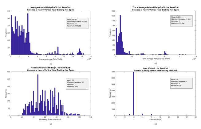
Figure 3.7: (a) AADT, (b) T-AADT, (c) Roadway Surface Width, and (d) Lane Width for Rear-End Crashes
