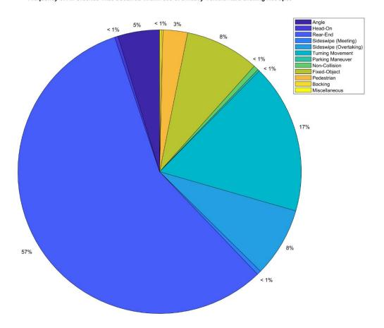
Frequency of All Crashes That Occurred Within 500 of a Heavy-Vehicle Hard Braking Hot Spot
